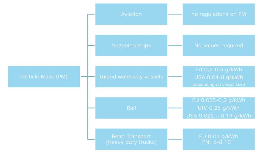
Source: VDMA, Exhaust emission legislation Diesel and gas engines
