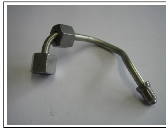
Pipe – Rail to Injector
