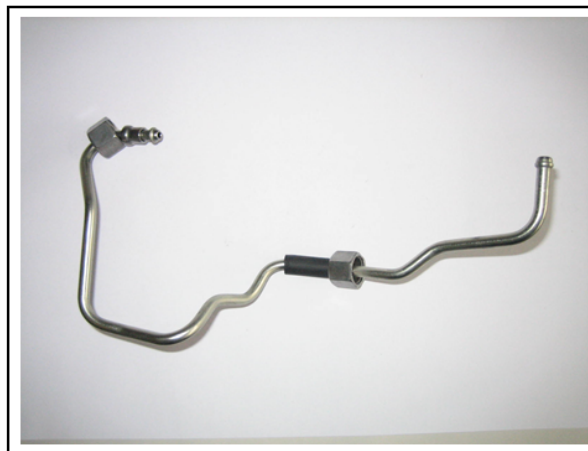
Pipe - Pump to Rail
