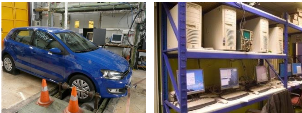
Figure 6: LAT chassis dyno (left) and chassis dyno control station (right)
