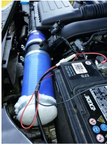
Figure 27: Extra MAF sensor
