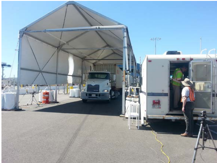
Figure 4. OHMS setting. The sampling pipe is located in the left corner of the tent; gas analyzers and other monitoring equipment are located in the mobile unit to the right. Courtesy: F. Posada
