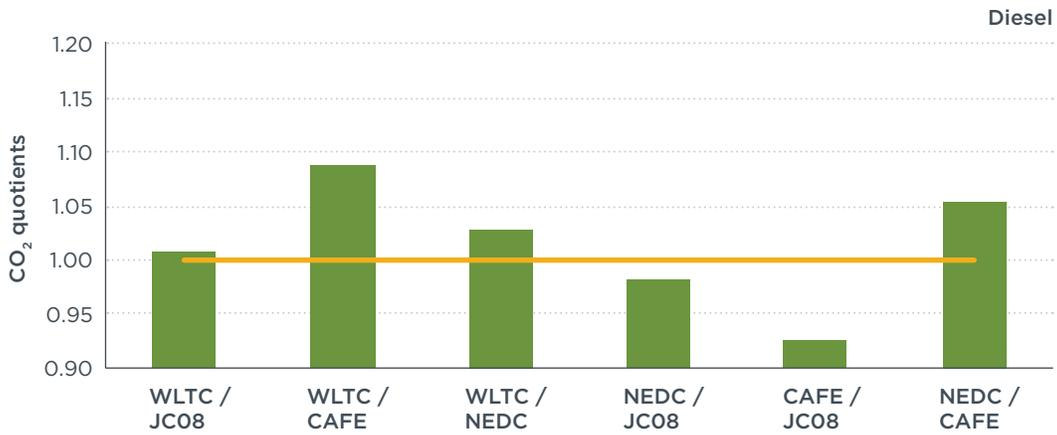
**Figure 8:** Cycle deviations of CO<sub>2</sub> emissions – averaged over all diesel technologies
