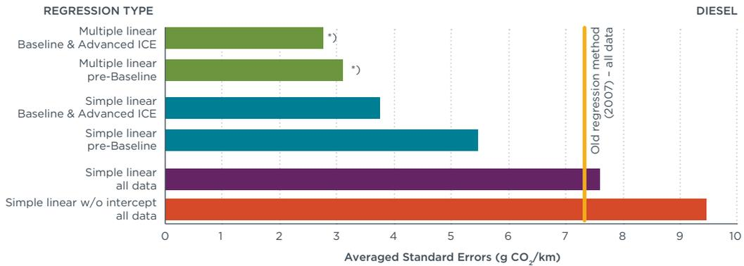
**Figure 10:** Standard deviations of single data points for diesel concepts — averaged over all cycle combinations
