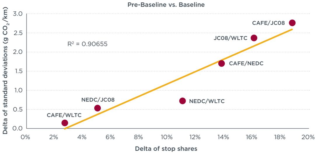
**Figure 11:** Difference of mean standard deviations between pre-Baseline and Baseline gasoline technologies depending on the differences of stop shares of the two cycles
