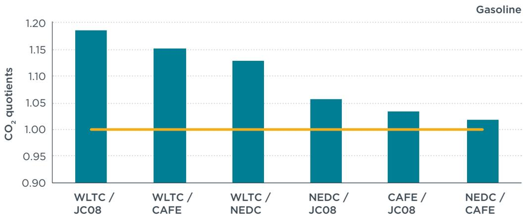
Figure 7: Cycle deviations of CO<sub>2</sub> emissions – averaged over all gasoline technologies
