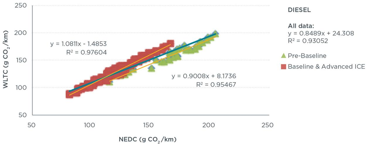
Figure C-10: Diesel regression results: WLTC over NEDC
