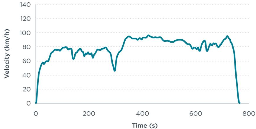
**Figure 2:** Driving schedule of the HWFET cycle
