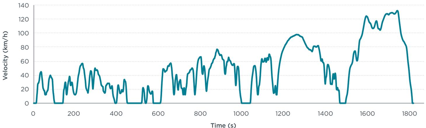
**Figure 5:** Driving schedule of the WLTC cycle (vehicle class 3, version 5)
