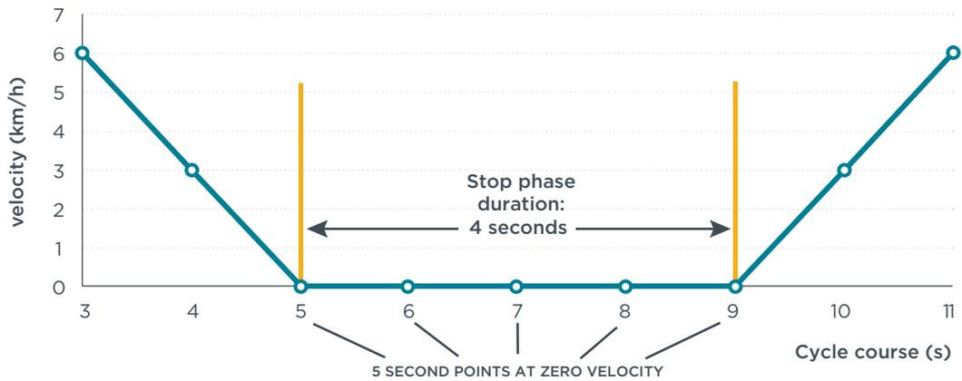
**Figure 6:** Example for the duration of a stop phase (= number of second points at zero velocity - 1)
