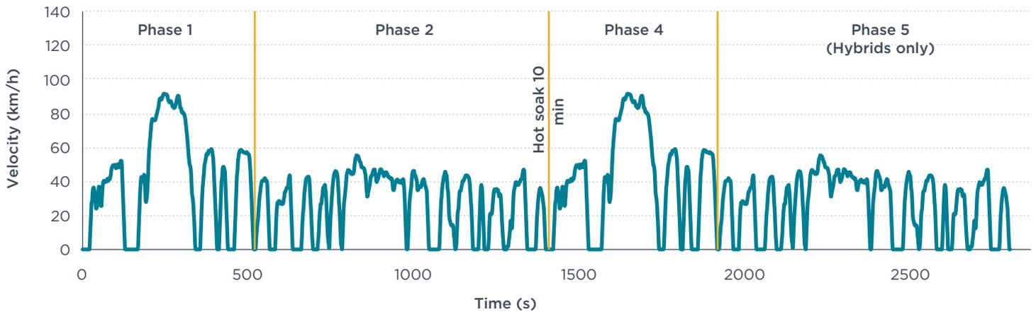
**Figure 1:** Driving schedule of the FTP75 cycle
