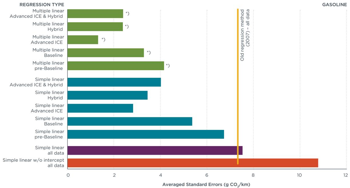
**Figure 9:** Standard deviations of single data points for gasoline concepts — averaged over all cycle combinations
