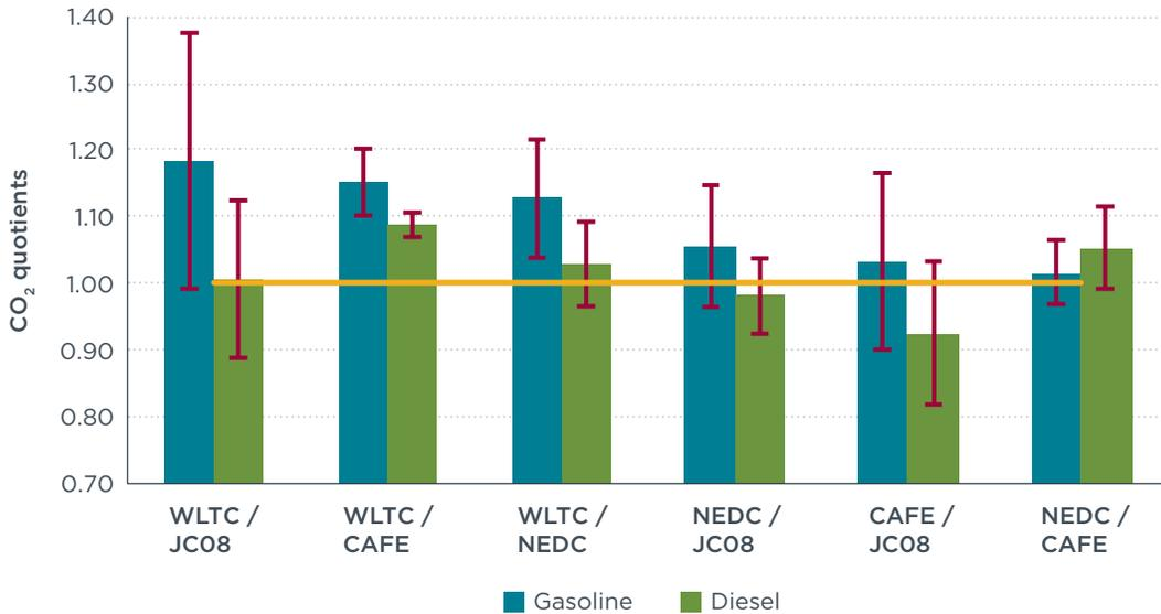
**Figure 12:** Averaged CO<sub>2</sub> emission quotients — results from basic single regression approach with zero intercept (approach no. 4 of Table 12). Error bars represent technology-specific standard deviations of single data points.
