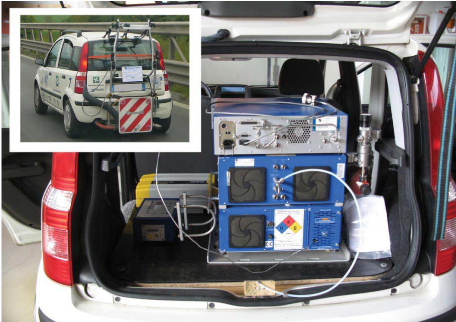
Figure 2: Passenger car instrumented with PEMS 2
