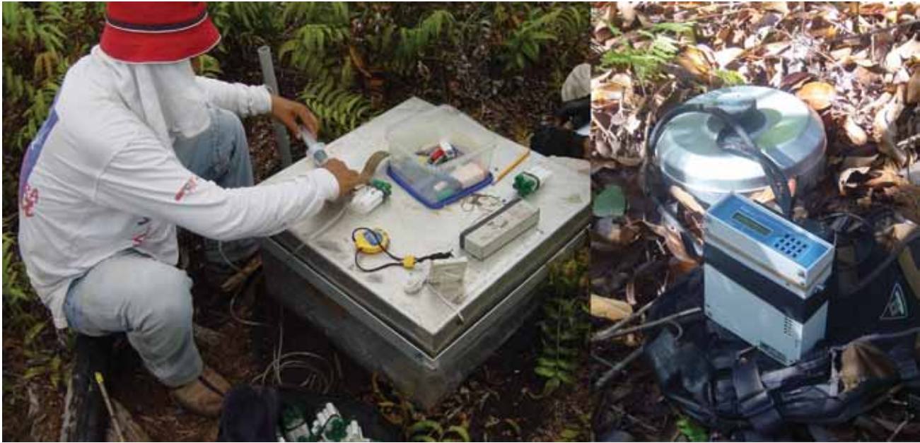
Figure 7: Closed chamber measurements being made in the field; large static chamber (left) and dynamic chamber and CO 2 analyzer (right; images: J. Jauhiainen).
