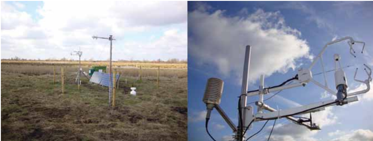
Figure 8: An eddy covariance flux tower measuring surface-atmosphere exchanges of CO 2 , water and energy at a restored fen peatland in the United Kingdom (left). Eddy covariance instrumentation, consisting of a sonic anemometer, an infrared gas analyzer, and sensors for measuring photosynthetically active radiation, air temperature and relative humidity (right). (Images: R. Morrison).
