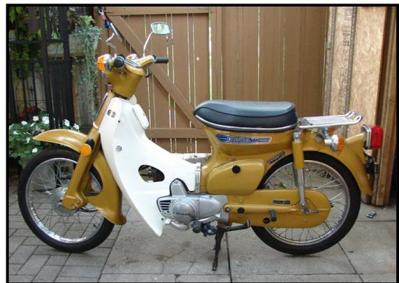
**Motorcycles:** Motorcycles perhaps do not need a detailed description since their constructional features are almost universal. They are constructed of metal frames; use an integrated power unit consisting of the engine, clutch, and gearbox and a final chain
