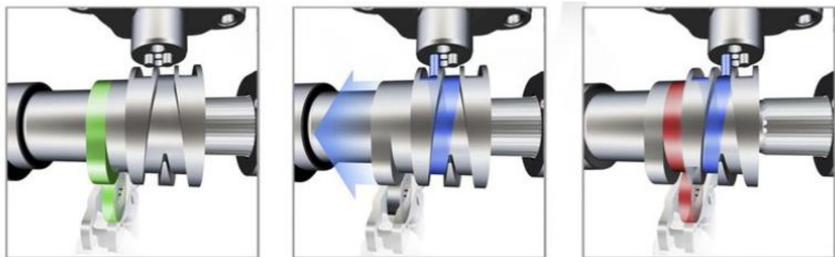
Figure 3.61 Functionality of the variable valve lift (Source: Volkswagen)
