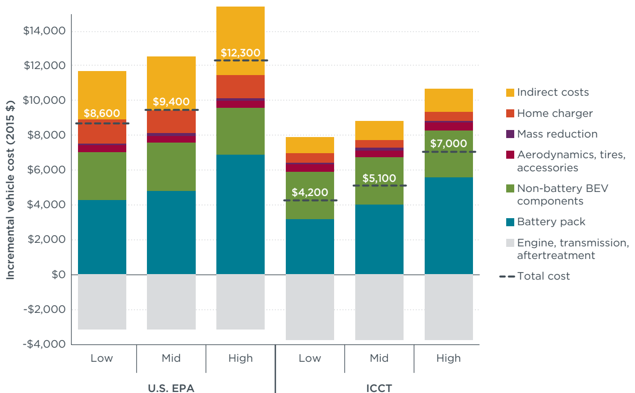
Figure 6. Battery electric vehicle cost in 2025 for low, mid, and high electric range vehicles based on U.S. EPA and ICCT data.
