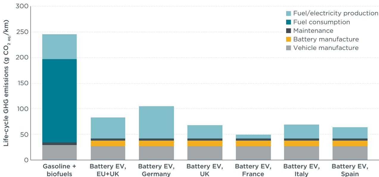
**Figure 3.5.** Life-cycle GHG emissions of lower medium segment BEVs registered in Europe in 2021, with the vehicle lifetime average electricity mix in the European Union and United Kingdom, Germany, United Kingdom, France, Italy and Spain, compared to gasoline ICEVs.
