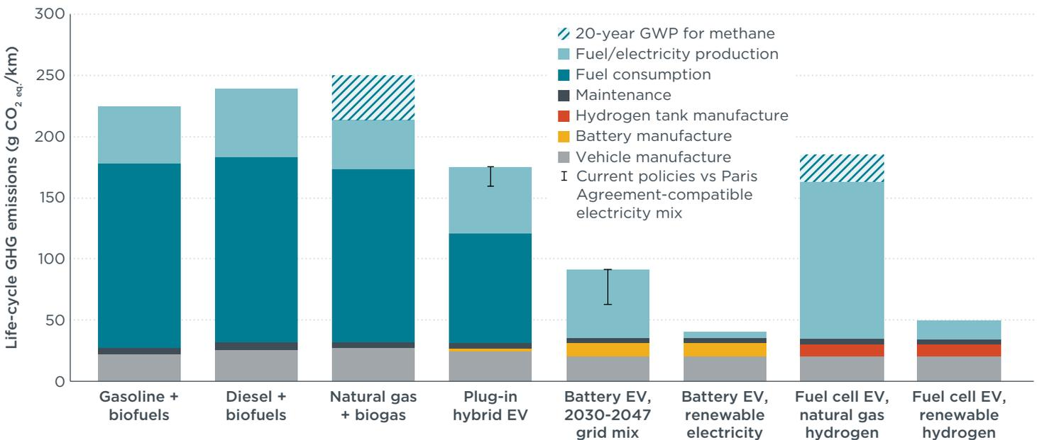
**Figure 7.2.** Life-cycle GHG emissions of average medium-size gasoline, diesel, and CNG ICEVs, PHEVs, BEVs, and FCEVs projected to be registered in China, Europe, India, and the United States in 2030.
