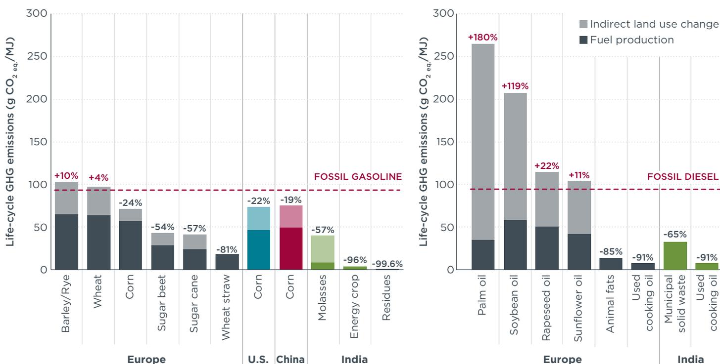
**Figure 7.5.** Production and indirect land use change emissions of the most relevant a) ethanol and b) biodiesel pathways considered in the gasoline and diesel blend in Europe, the United States, China, and India, compared to the production and combustion emissions of fossil gasoline and diesel.
