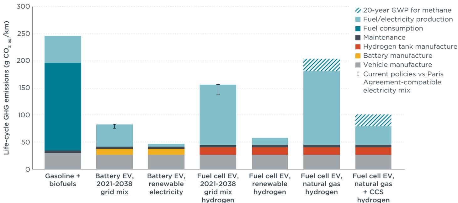
**Figure 3.6.** Life-cycle GHG emissions of 2021 lower medium car segment BEVs and FCEVs using the EU average electricity mix or only renewable electricity and FCEVs using natural gas derived hydrogen with and without CCS, compared to gasoline ICEVs.
