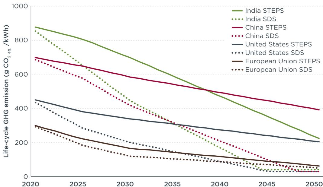
**Figure 2.1.** Life-cycle GHG emissions of electricity consumption based on an electricity mix of IEA's Stated Policy (STEPS) and Sustainable Development Scenario (SDS), the IPCC's life-cycle GHG emission factors, and energy losses in the grids.
