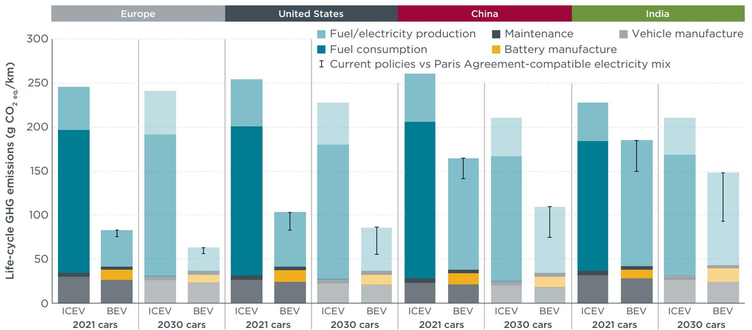
**Figure ES.1.** Life-cycle GHG emissions of average medium-size gasoline internal combustion engine (ICEVs) and battery electric vehicles (BEVs) registered in Europe, the United States, China, and India in 2021 and projected to be registered in 2030. The error bars indicate the difference between the development of the electricity mix according to stated policies (the higher values) and what is required to align with the Paris Agreement.
