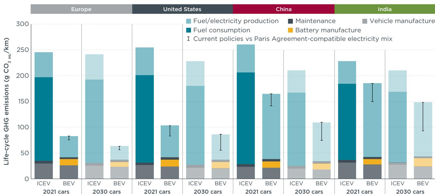
**Figure 7.3.** Life-cycle GHG emissions of average medium-size gasoline ICEVs and BEVs. The error bars indicate the difference between the development of the electricity mix according to the IEA’s Stated Policy Scenario or Sustainable Development Scenario.
