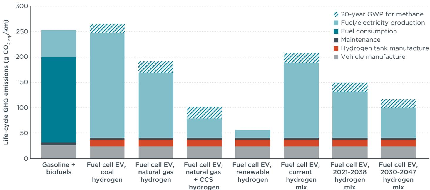
**Figure 7.4.** Life-cycle GHG emissions of global typical medium-size FCEVs powered by coal-, natural gas-, CCS natural gas-, or renewable electricity-based hydrogen, by the current mix of these pathways and by the expected lifetime average mix for cars registered in Europe, the United States, China, and India in 2021 and in 2030, compared to global typical gasoline cars registered in 2021.
