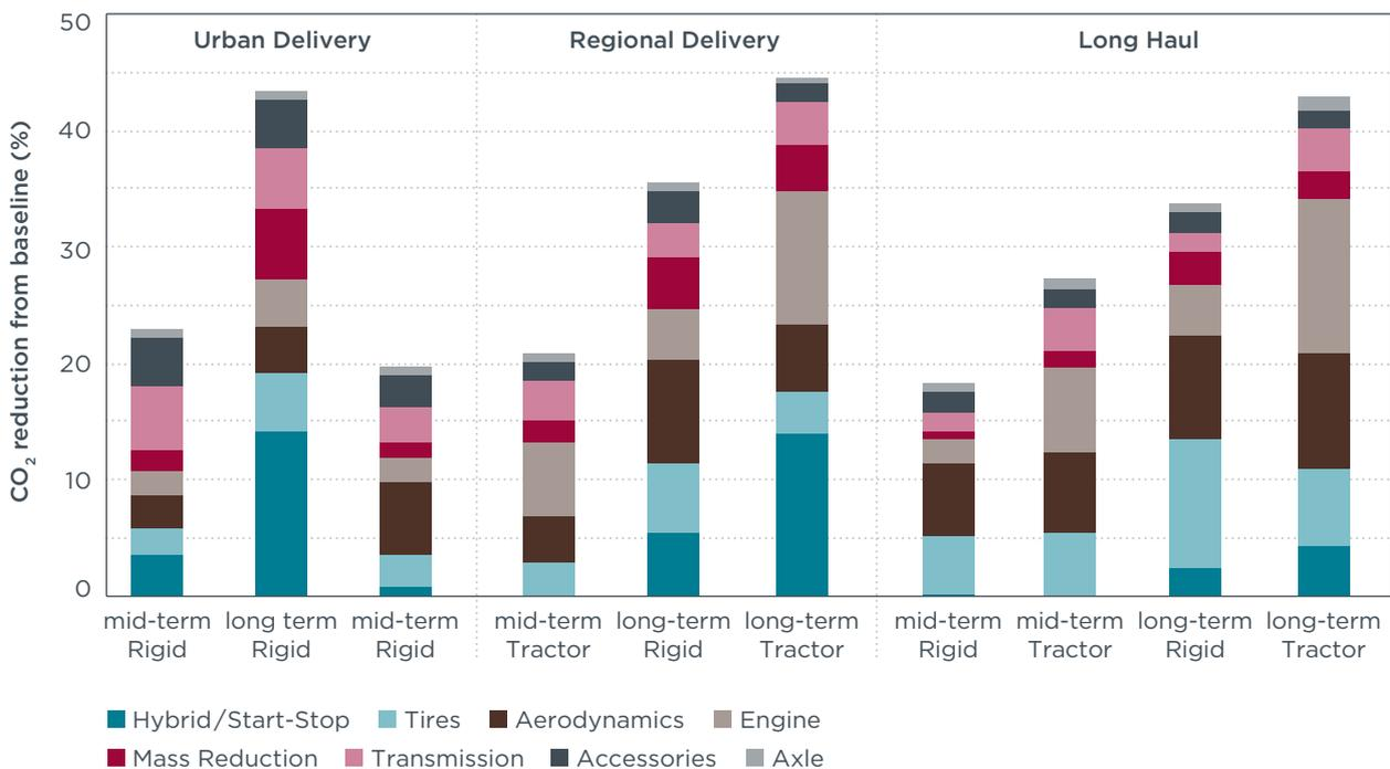
**Figure 1.** There is significant technology potential to improve the fuel-efficiency and reduce the CO<sub>2</sub> emissions of the average freight truck in the EU in both the mid-term (now to 2025) and long term (2030).
