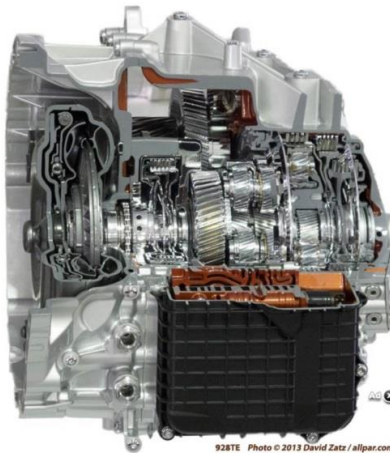
Image 2: ZF 9-Speed Automatic Transmission for Chrysler and Dodge Cars (Source: http://www.allpar.com/mopar )
