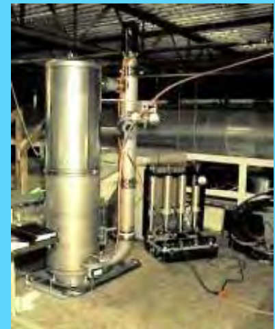
Cooking emission sampling atop laboratory cookstoves
