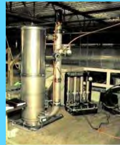
Cooking emission sampling atop laboratory cookstoves
