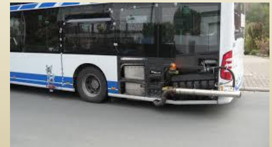
Field measurement with PEMS
