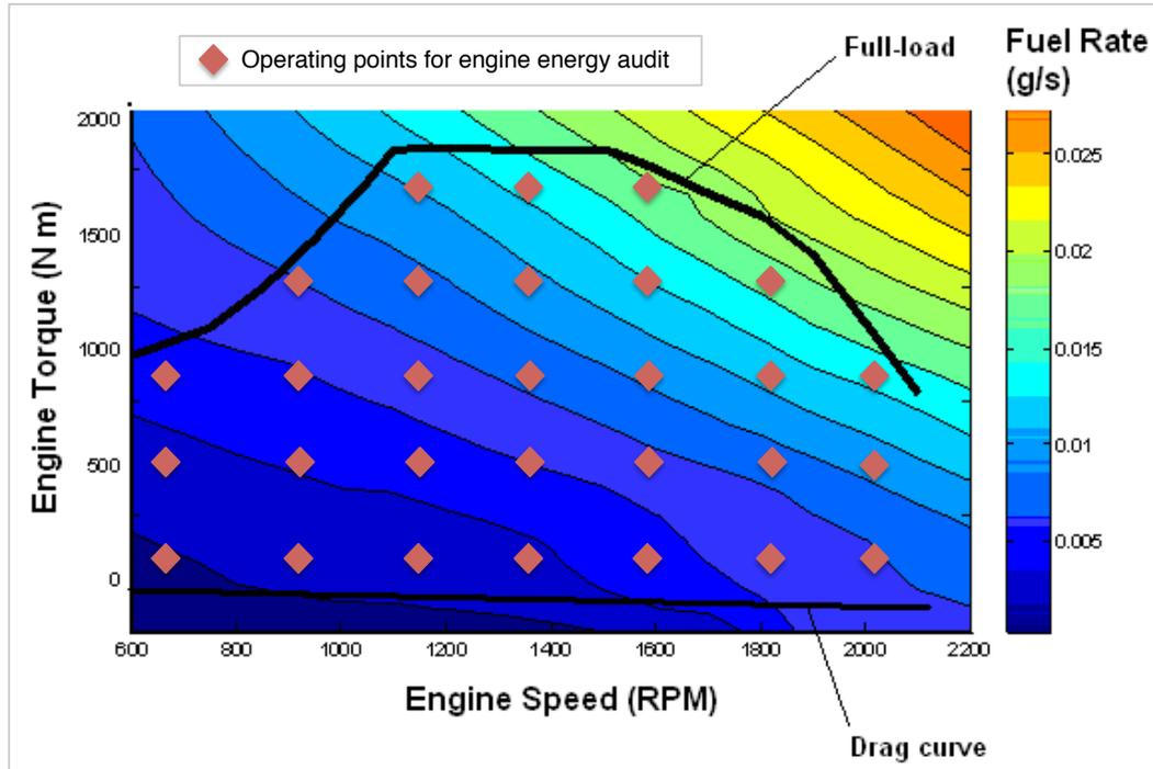
**Figure 3. Illustration of operating points on engine map that are chosen for energy audit in Task 2**
