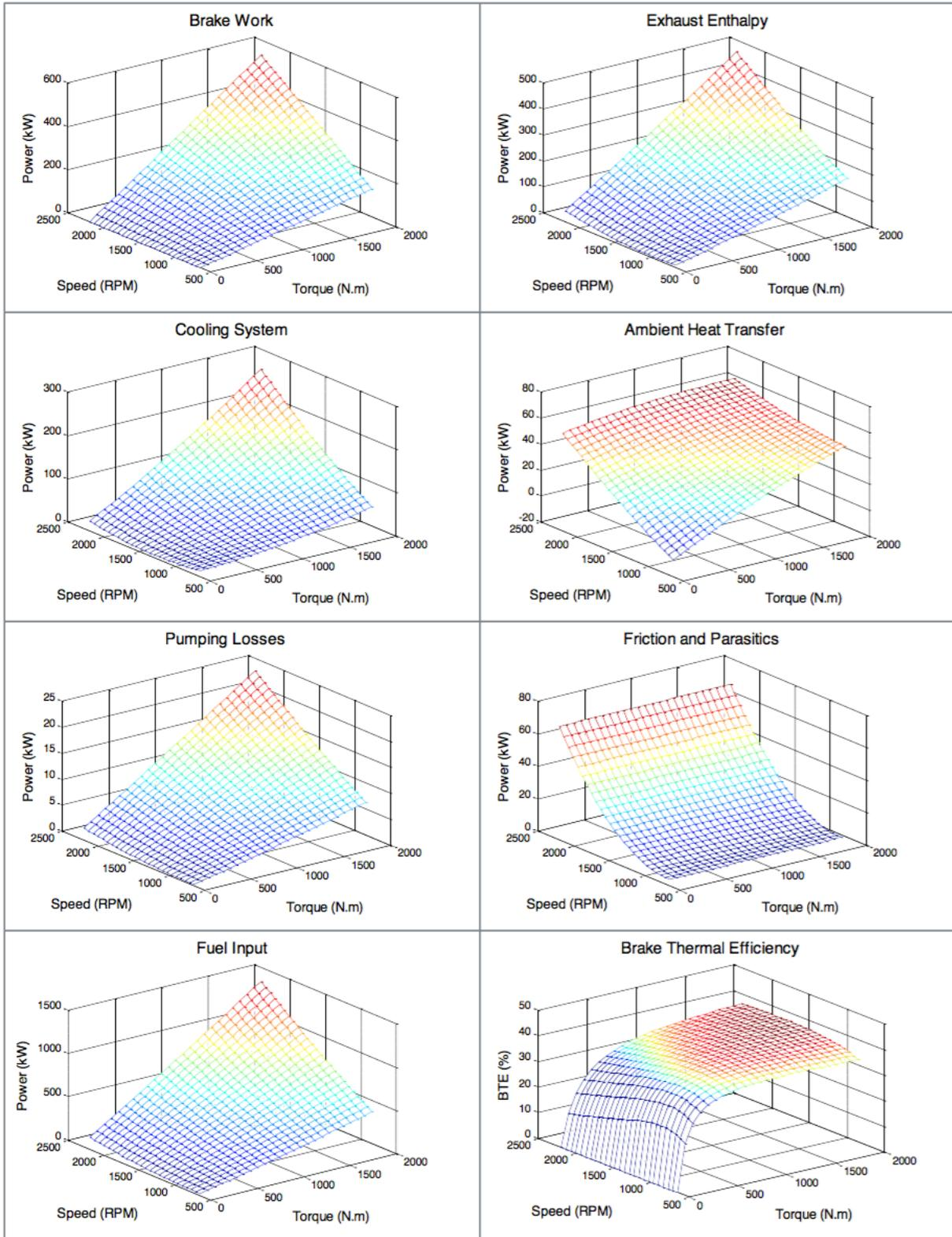
**Figure 4: engine energy flows, fuel input, and brake-specific fuel efficiency**
