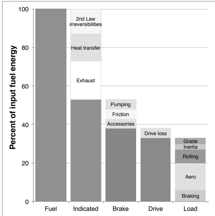
**Figure 2. Illustration of vehicle energy audit output**
