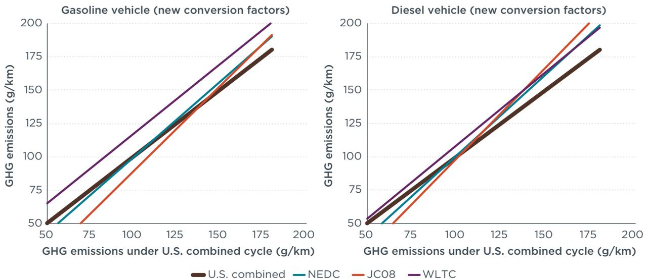
**Figure 1.** Relative stringency of the four test cycles (gasoline and diesel)
