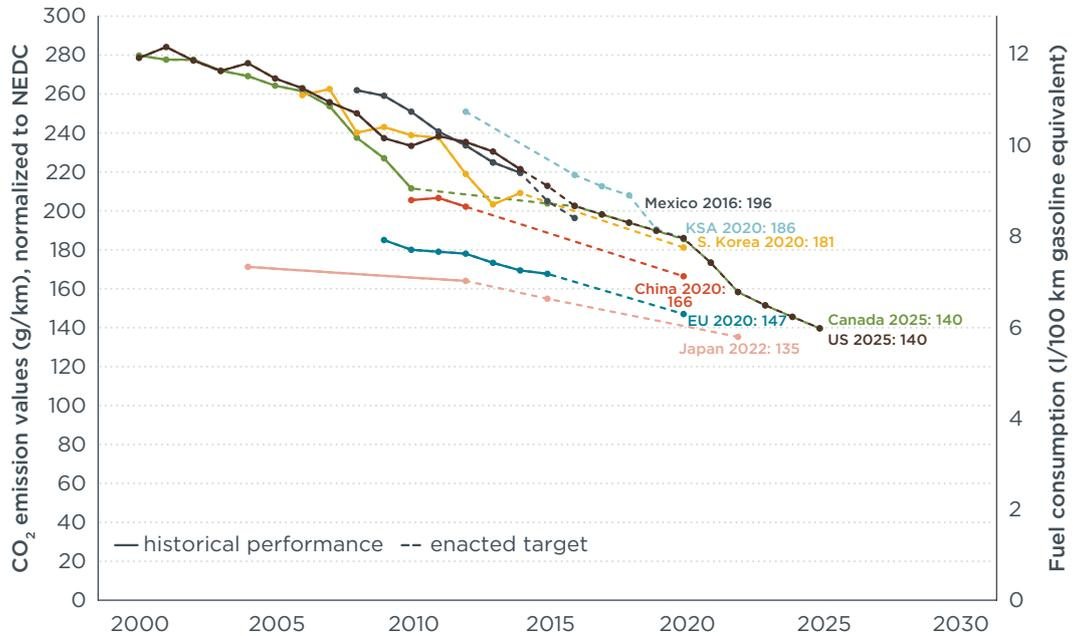
**Figure 3.** Historical fleet CO<sub>2</sub> emissions performance and current standards (gCO<sub>2</sub>/km normalized to NEDC) for LCVs
