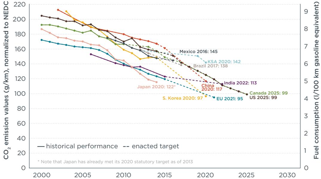
**Figure 2.** Historical fleet CO<sub>2</sub> emissions performance and current standards (gCO<sub>2</sub>/km normalized to NEDC) for passenger cars
