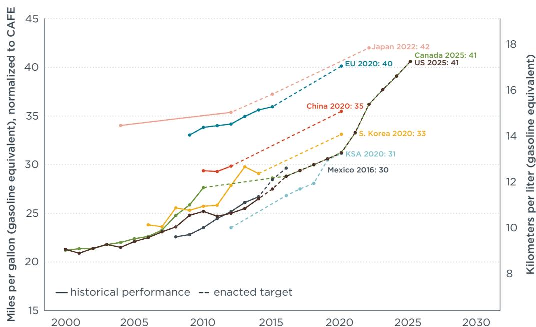
**Figure 5.** Historical fleet CO<sub>2</sub> emissions performance and current standards (mpg normalized to U.S. CAFE test cycles) for LCVs
