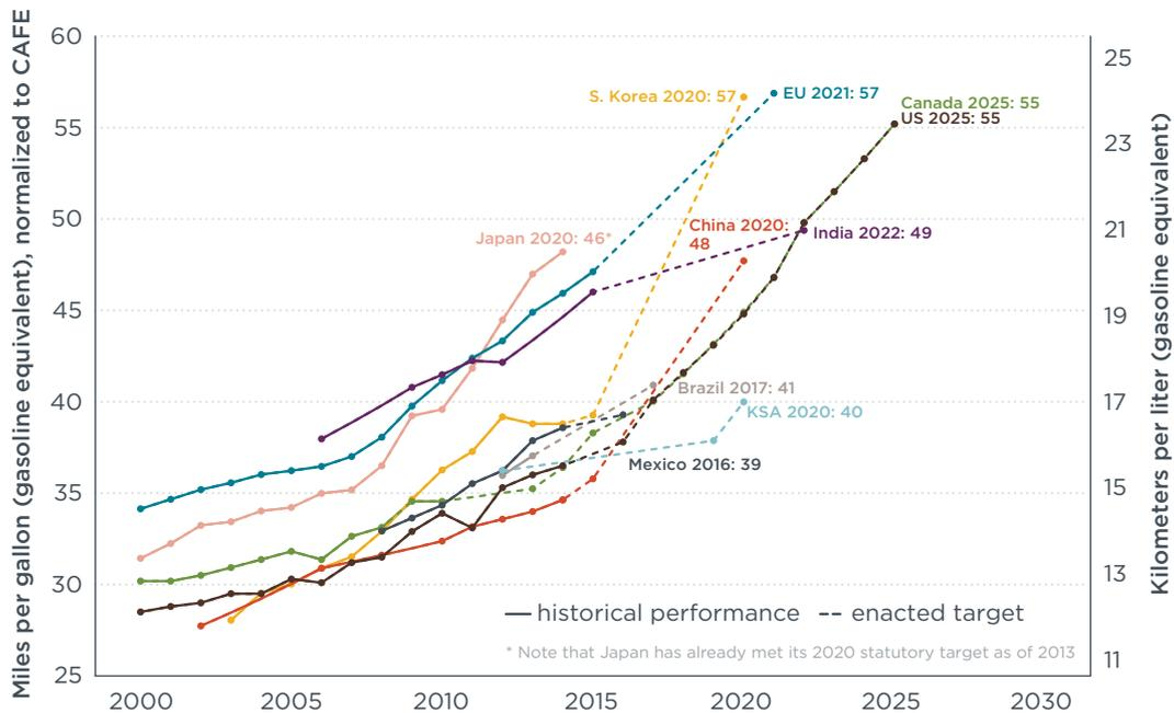
**Figure 4.** Historical fleet CO<sub>2</sub> emissions performance and current standards (mpg normalized to U.S. CAFE test cycles) for passenger cars
