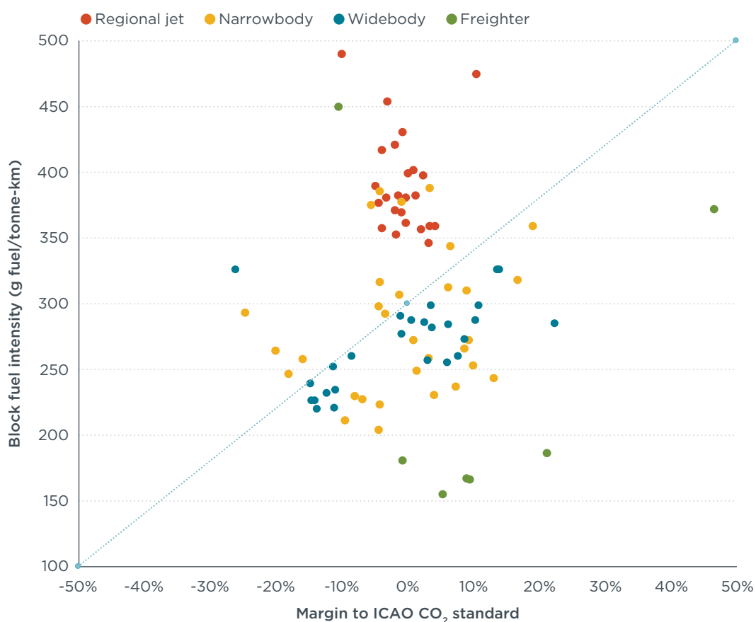
Figure 8. Margin to ICAO's CO 2 standard versus block fuel intensity of new aircraft by type for EIS 2000 to 2020 planes.
