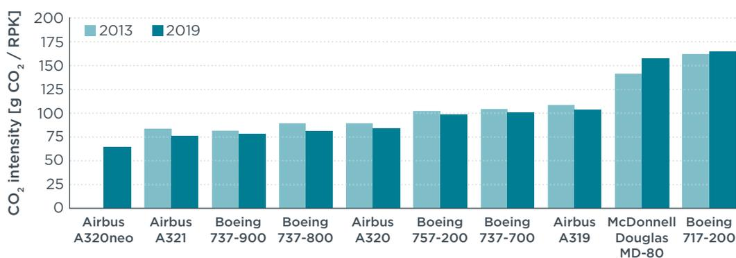
**Figure 7.** Passenger CO<sub>2</sub> intensity of the top 10 highest emitting narrowbody aircraft types, 2013 and 2019
