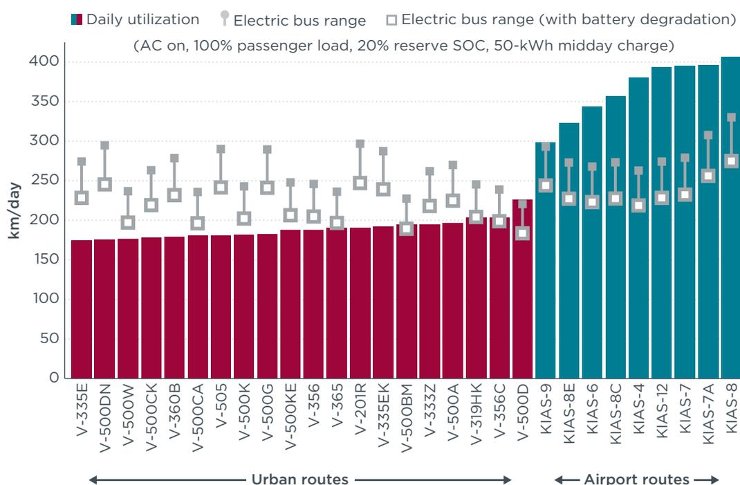
**Figure 17.** Estimated range under new and aged battery conditions by route with midday charging, compared with average route-level daily utilization of the existing diesel fleet.
