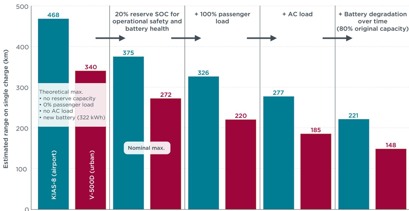
**Figure 15.** Impacts of key variables on estimated driving range for electric buses operating on selected BMTC routes.
