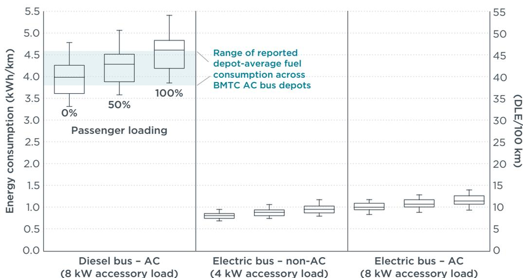
**Figure 12.** Energy consumption estimates for all modeling scenarios. The right axis shows fuel consumption in terms of the energy equivalent of a liter of diesel fuel, referred to as diesel liter equivalent (DLE).
