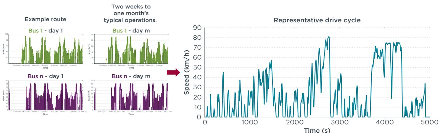
**Figure 11.** Illustration of a drive cycle developed for a route from real-world operational data.
