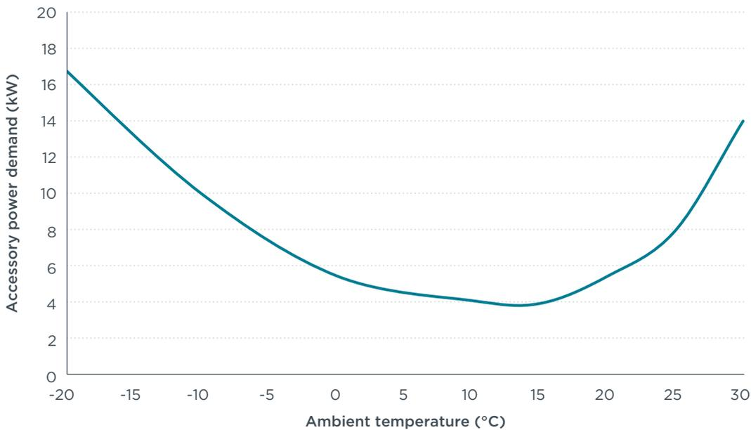
**Figure 2.** Accessory power consumption as a function of ambient temperature. Adapted from Klaus Kivekäs et al., “City Bus Powertrain Comparison: Driving Cycle Variation and Passenger Load Sensitivity Analysis,” *Energies* 11, no. 7 (2018): 11, 1755, <https://doi.org/10.3390/en11071755>, and Antti Lajunen and Kari Tammi, “Energy Consumption and Carbon Dioxide Emission Analysis for Electric City Buses,” in *International Electric Vehicle Symposium and Exhibition*, Montreal, Canada (2016): 1–12.
