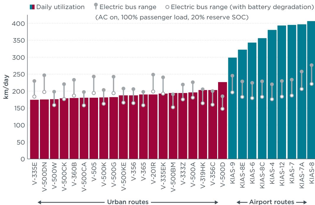
**Figure 16.** Estimated range under new and aged battery conditions by route compared to average route-level daily utilization of the existing diesel fleet.
