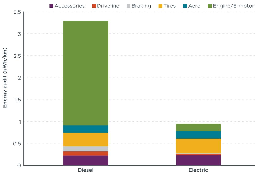
**Figure 4.** Energy audit in absolute units for diesel and electric buses over the World Harmonized Vehicle Cycle-India cycle with 50% passenger load and AC on.
