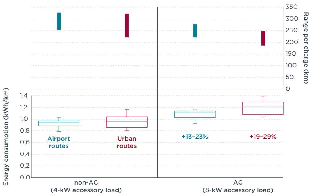
**Figure 14.** Impacts of accessory load on energy consumption and electric bus range estimates. 100% passenger load conditions are assumed. Range calculations assume a 322-kWh battery capacity and a 20% reserve SOC (i.e., 258-kWh usable capacity). Percentages indicate the change in median energy consumption estimates relative to the 4-kW accessory load scenario.
