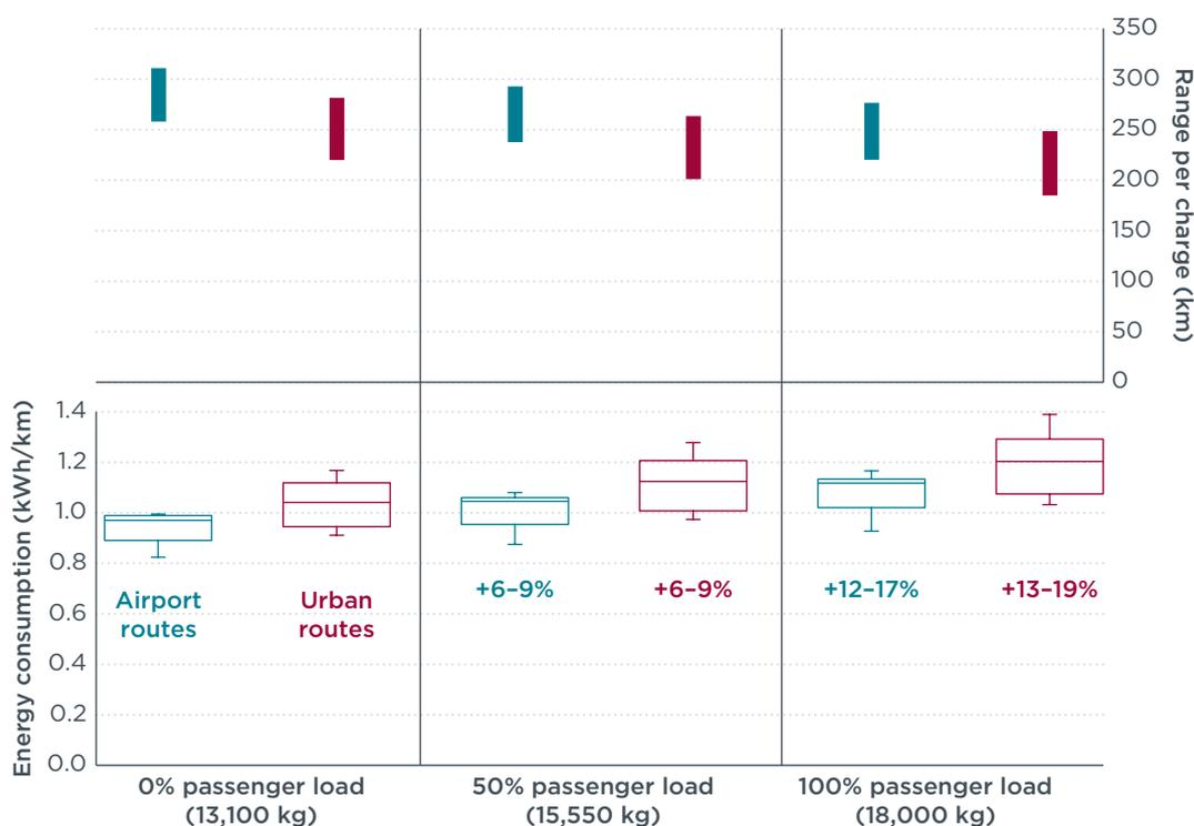
**Figure 13.** Impacts of passenger load assumptions on energy consumption and electric bus range estimates. An 8-kW accessory power consumption is assumed (i.e., AC on). Range calculations assume a 322-kWh battery capacity and a 20% reserve SOC (i.e., 258-kWh usable capacity). Percentages indicate change in energy consumption estimates relative to the 0% load scenarios.
