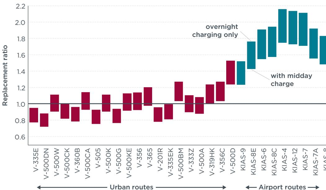
**Figure 18.** Electric bus replacement ratio estimates for 29 BMTC routes.
