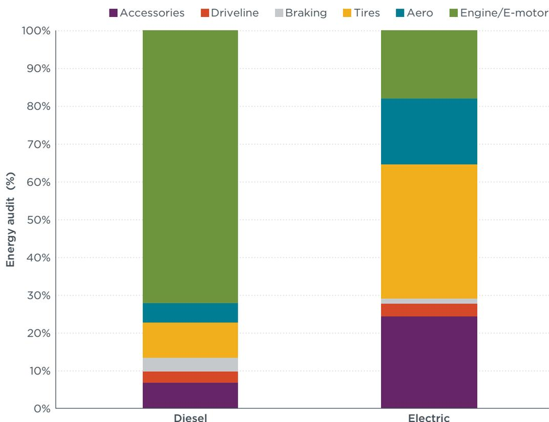
**Figure 5.** Energy audit (relative) for diesel and electric buses over the World Harmonized Vehicle Cycle-India cycle, with 50% passenger load and AC on.
