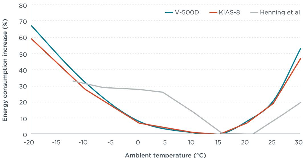
**Figure 3.** Energy consumption increase as a function of ambient temperature.
