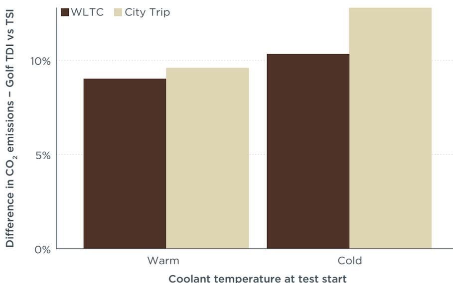
**Figure 13.** Comparison of the relative difference in cycle CO<sub>2</sub> emissions of the Golf TDI and Golf TSI for both a cold- and warm-start WLTC at 23 °C and a test with a representative duration and distance for trips performed by the German urban population.
