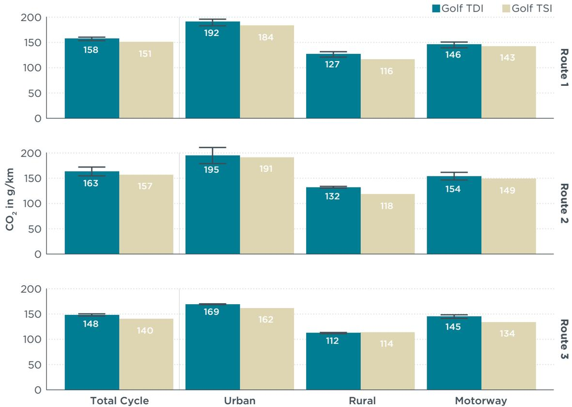
**Figure 14.** Real-world driving – CO<sub>2</sub> emissions of the Golf TDI and Golf TSI for tests performed on three different routes. The bars show the average value for all tests performed with the same vehicle on one route. The error bars show the minimum to maximum range of results if multiple tests were performed on one route. No error bar is shown if only one test was performed. The Golf TDI tests on Route 3 were corrected for the particulate filter regeneration.
