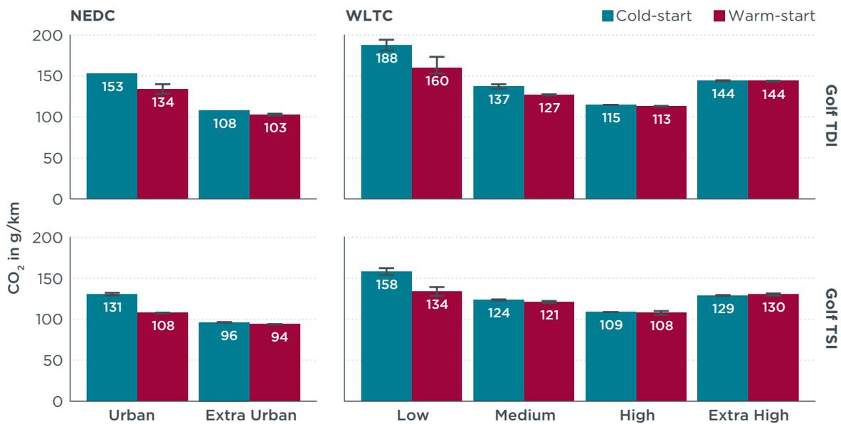
**Figure 8.** Comparison of phase CO<sub>2</sub> emission levels—Cold- versus warm-start NEDC and WLTC at 23°C. The error bar shows the minimum to maximum range of results if multiple tests were performed. No error bar is shown if only one test was performed.
