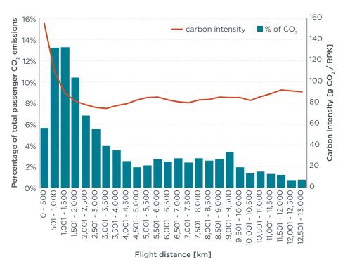
Figure 3. Share of passenger CO<sub>2</sub> emissions and carbon intensity in 2018, by stage length.
