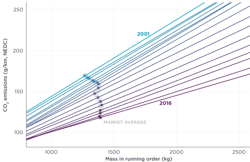
Figure 4. Relation between CO 2 emissions and vehicle mass in 2001–2016 based on sales-weighted linear regression analyses. Round markers denote average mass and CO 2 emissions of new vehicles in each year.
