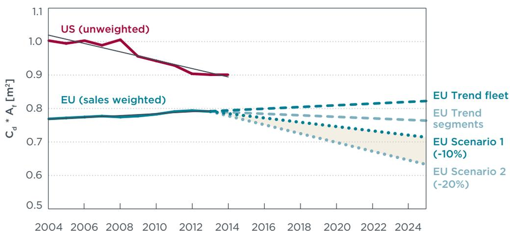
**Figure 16.** Aerodynamic drag: 10-year trends with U.S. and EU and projections to 2025.
