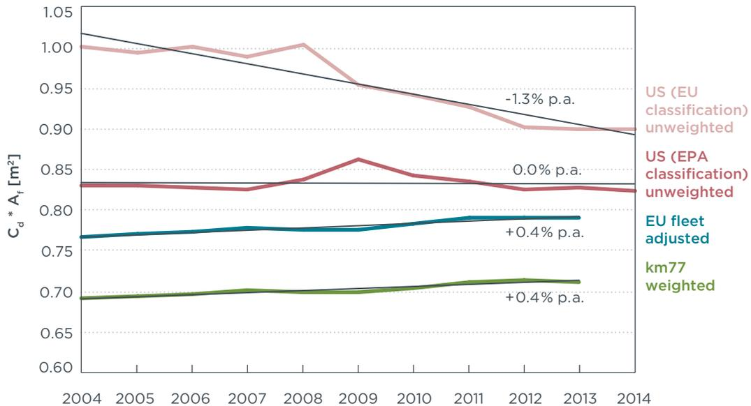
**Figure 10.** Aerodynamic drag – 10-year trend of cars’ fleet averages, showing U.S. unweighted values based on EU classification with all SUVs, U.S. unweighted values based on EPA classification without heavy SUVs, select weighted EU data from the km77 database, and EU values adjusted to realistic fleet averages.
