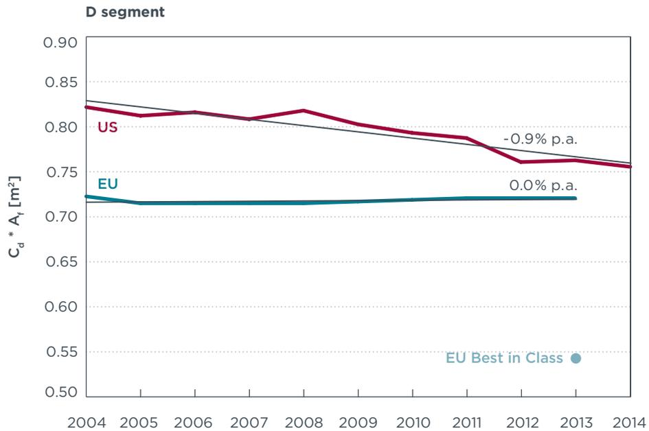
**Figure C-4.** Aerodynamic drag of D segment cars in the EU and U.S. - Annual averages of the past 10 years and actual best-in-class model.
