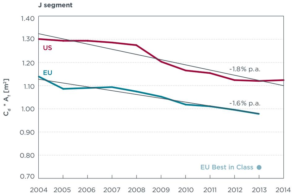
**Figure C-6.** Aerodynamic drag of J segment cars in the EU and U.S. – Annual averages of the past 10 years and actual best-in-class model.
