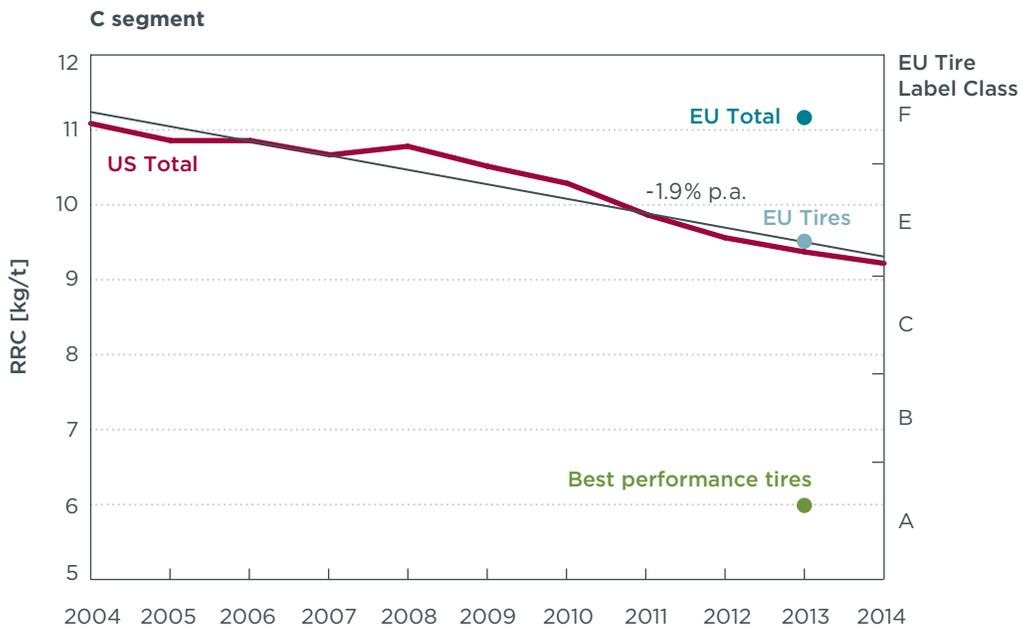
**Figure B-2.** Vehicle rolling resistance of C segment cars – Annual averages of the past 10 years in the U.S. and actual EU averages (total vehicle and tires only).
