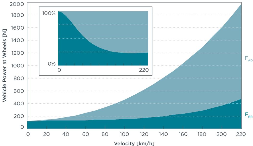
**Figure 3.** Typical distribution of rolling resistance force ( $F_{RR}$ ) and aerodynamic drag force ( $F_{AD}$ ) over vehicle velocity.
