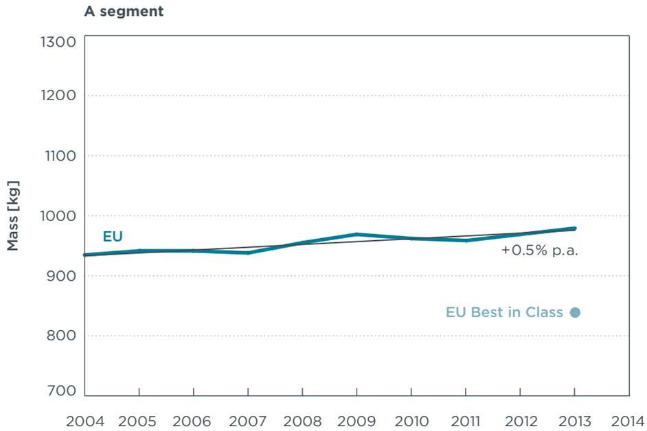
**Figure A-1.** Vehicle mass of A segment cars in the EU – Annual averages of the past 10 years and actual best-in-class model.
