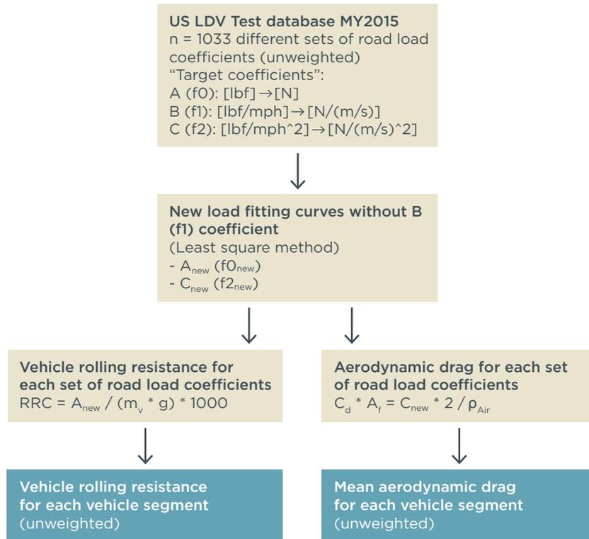
**Figure 7.** Scheme for calculating the segment-specific rolling resistance coefficients and aerodynamic drags from the US EPA LDV certification database.
