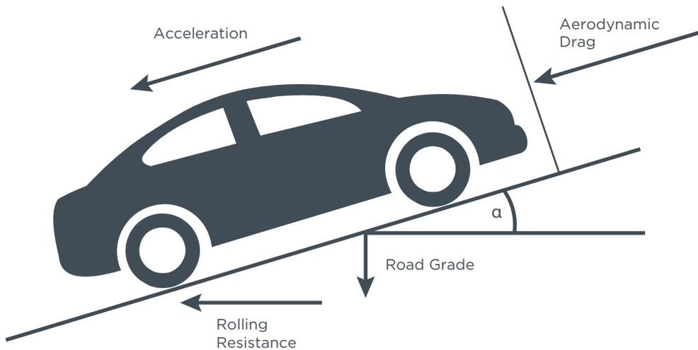
**Figure 1.** Resistance forces affecting a moving vehicle.
