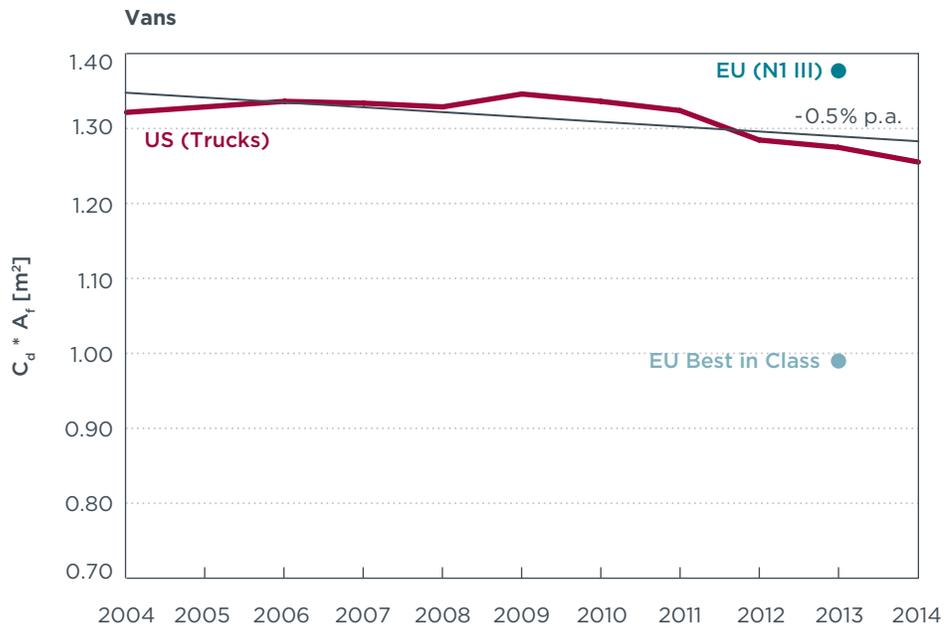
**Figure C-7.** Aerodynamic drag of vans in the EU and U.S. – Annual averages of the past 10 years and actual best-in-class model.
