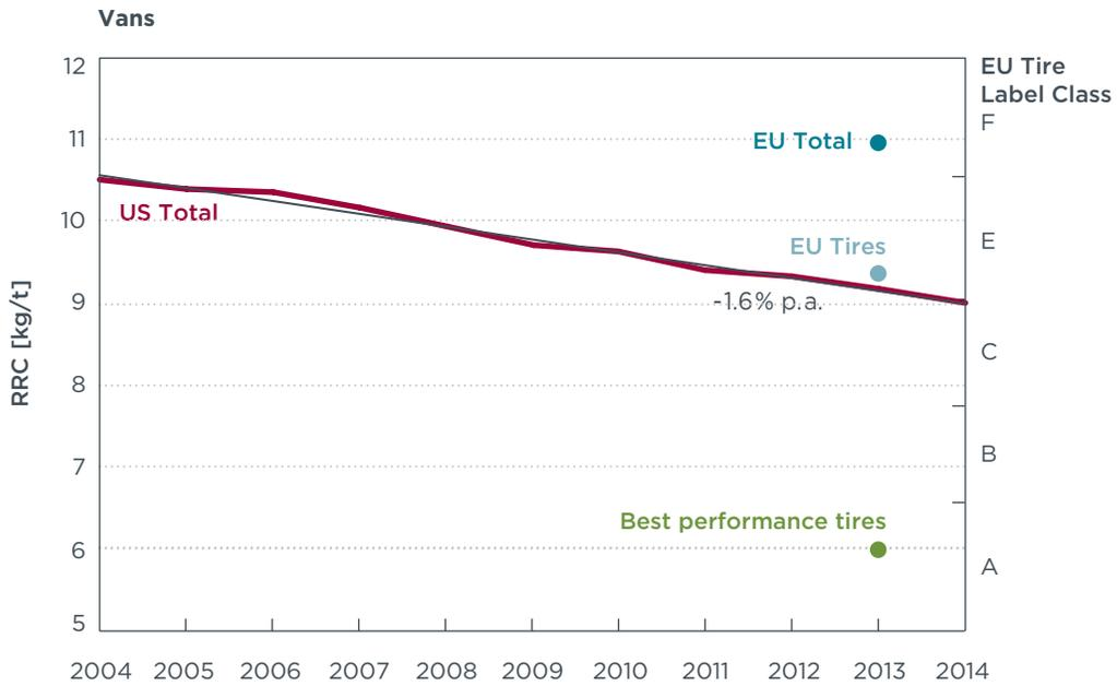
**Figure B-6.** Vehicle rolling resistance of vans – Annual averages of the past 10 years in the U.S. and actual EU averages (total vehicle and tires only).
