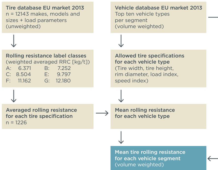
**Figure 6.** Scheme illustrating the derivation of volume-weighted and segment-specific tire rolling resistance coefficients. (RRC label class D not applied for LDV tires.)
