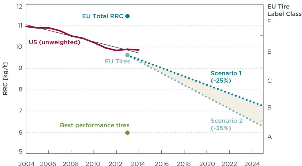
**Figure 15.** Rolling resistance: 10-year trend U.S. (total rolling resistance), status quo EU (total and tires only) and projections to 2025.
