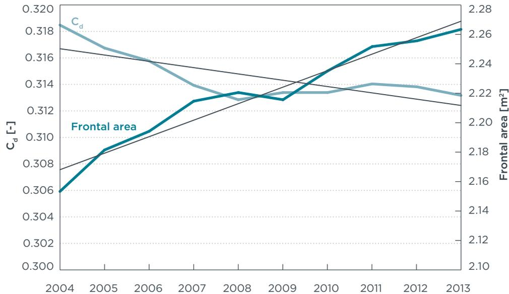
**Figure 11.** 10-year trends for EU aerodynamic drag coefficients and frontal areas of new passenger cars – Fleet averages using data from km77 database and not adjusted to realistic fleet averages.
