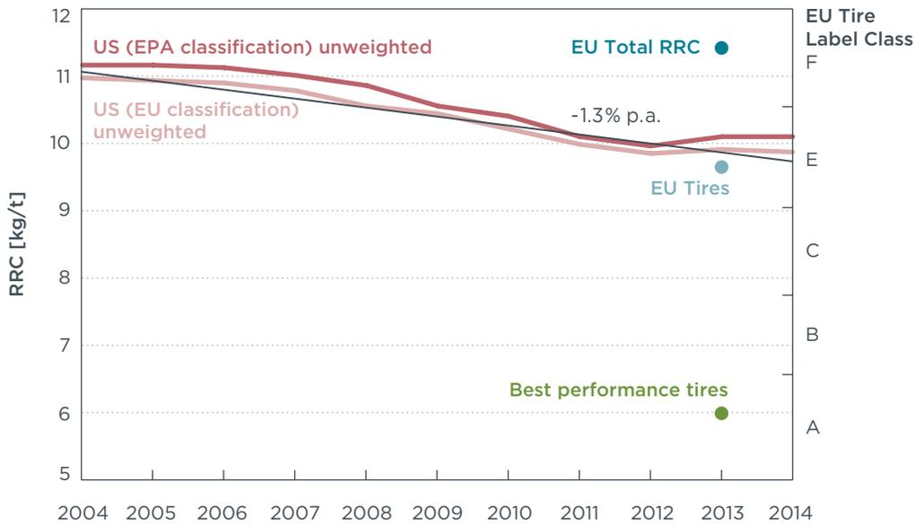
**Figure 9.** Rolling resistance: 10-year trend U.S. car fleet (whole vehicle), EU classification with all SUVs, EPA classification without heavy SUVs, and status quo EU (total and tires only).
