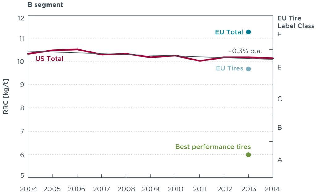
**Figure B-1.** Vehicle rolling resistance of B segment cars - Annual averages of the past 10 years in the U.S. and actual EU averages (total vehicle and tires only).
