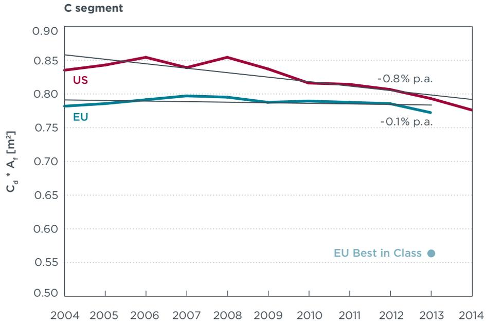
**Figure C-3.** Aerodynamic drag of C segment cars in the EU and U.S. - Annual averages of the past 10 years and actual best-in-class model.
