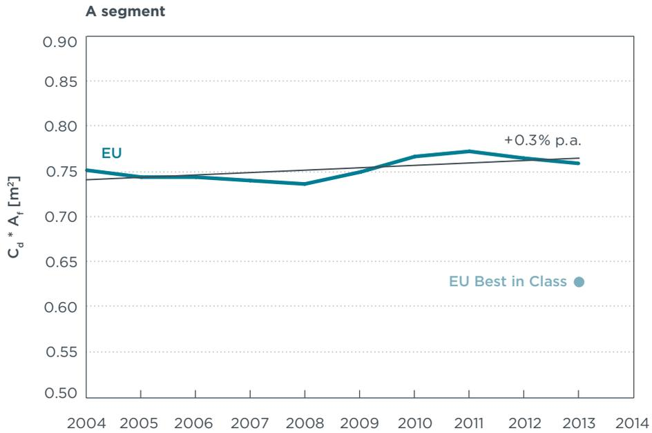
**Figure C-1.** Aerodynamic drag of A segment cars in the EU - Annual averages of the past 10 years and actual best-in-class model.
