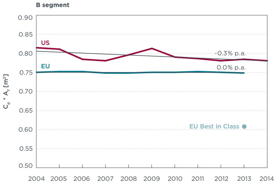
**Figure C-2.** Aerodynamic drag of B segment cars in the EU and U.S. - Annual averages of the past 10 years and actual best-in-class model.
