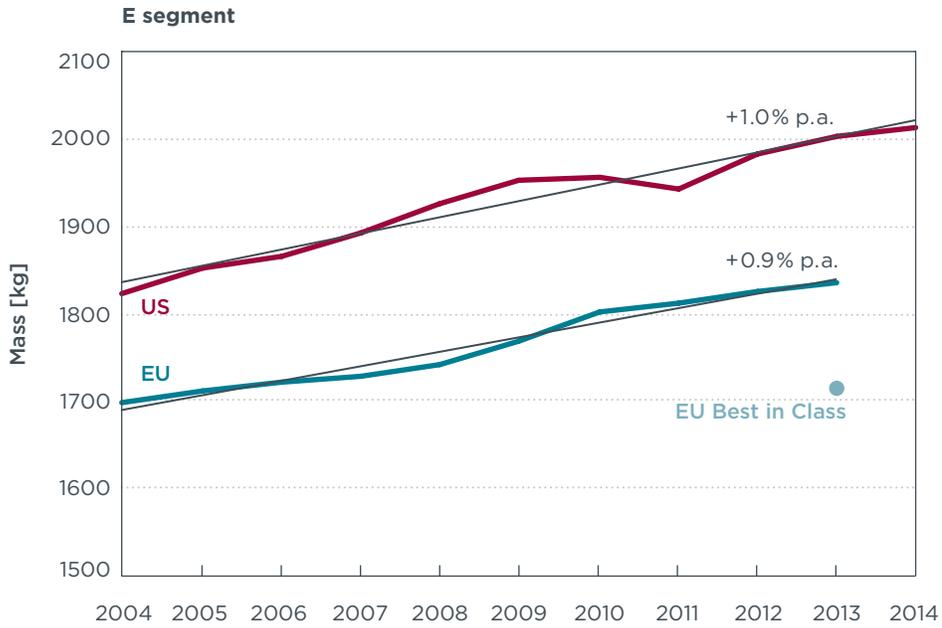
**Figure A-5.** Vehicle mass of E segment cars in the EU and U.S. - Annual averages of the past 10 years and actual best-in-class model.
