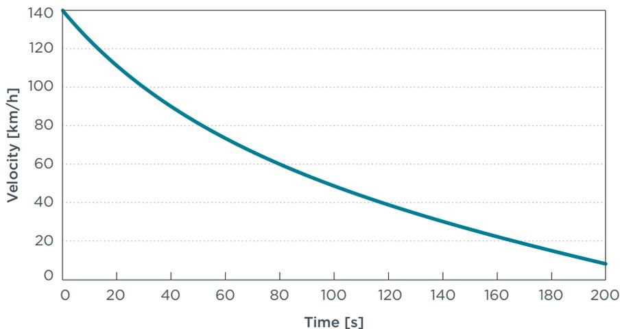
**Figure 2.** Typical course of vehicle's velocity during coast down (gearbox in neutral).
