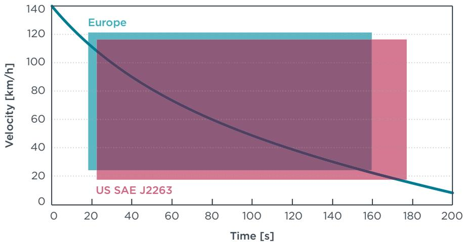
**Figure 4.** EU and U.S. velocity ranges of coastdown runs (EU interval averages).
