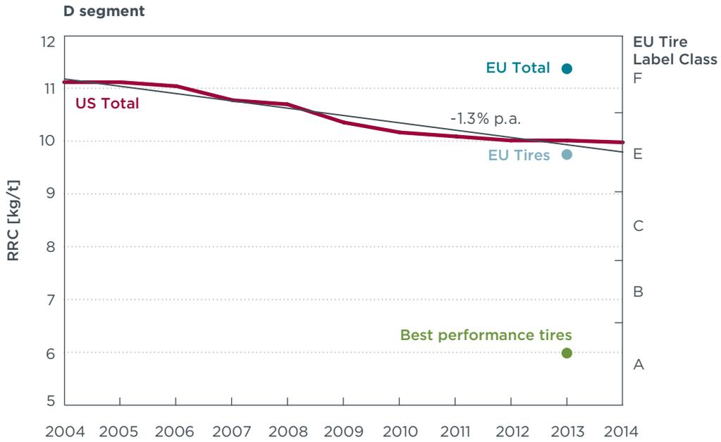
**Figure B-3.** Vehicle rolling resistance of D segment cars – Annual averages of the past 10 years in the U.S. and actual EU averages (total vehicle and tires only).
