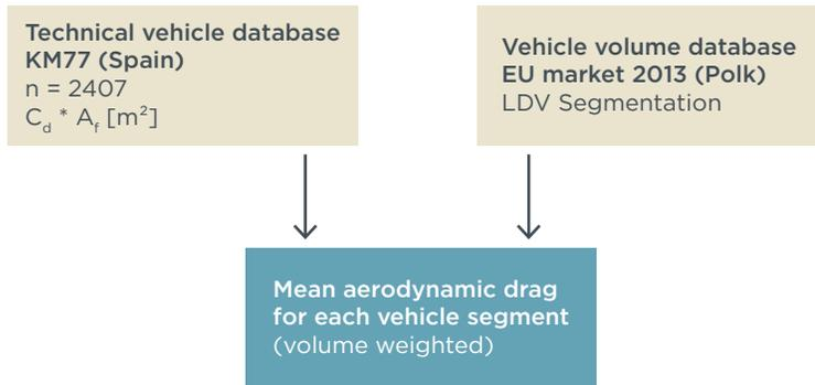
**Figure 5.** Scheme for the calculation of volume weighted and segment-specific aerodynamic drags ( $C_d * A_f$ ).
