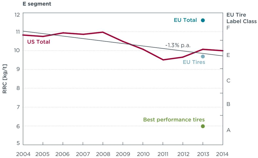
**Figure B-4.** Vehicle rolling resistance of E segment cars – Annual averages of the past 10 years in the U.S. and actual EU averages (total vehicle and tires only).
