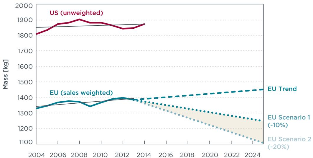
**Figure 13.** Projected mass market averages for cars, based on 10-year trend U.S. (test masses) and EU (mass in running order) and technical projections EU to 2025.
