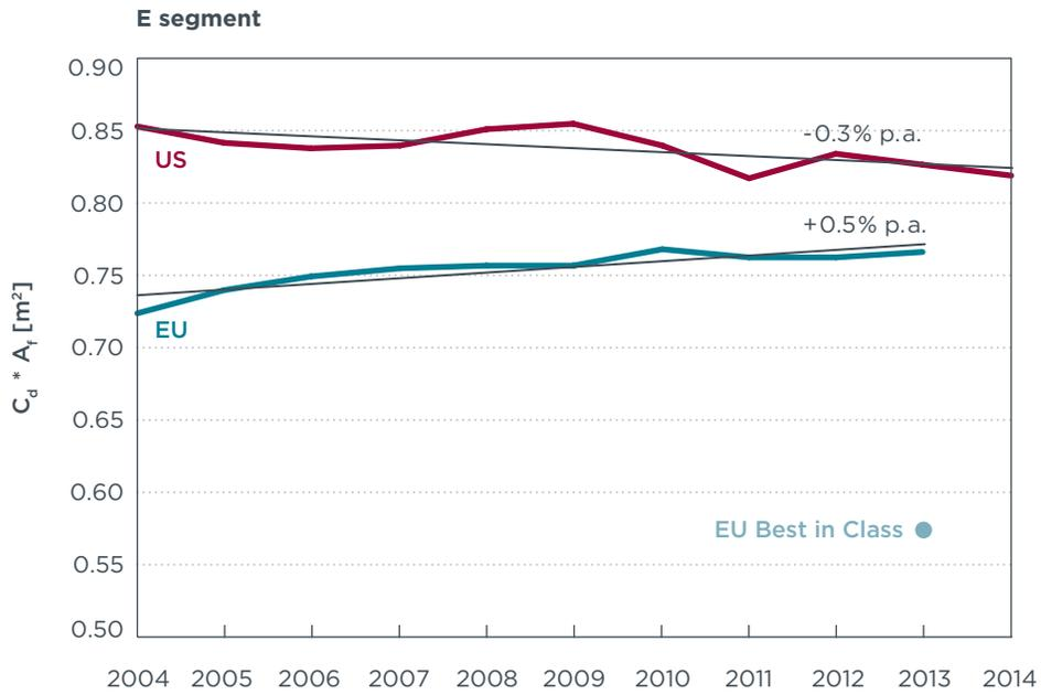
**Figure C-5.** Aerodynamic drag of E segment cars in the EU and U.S. – Annual averages of the past 10 years and actual best-in-class model.
