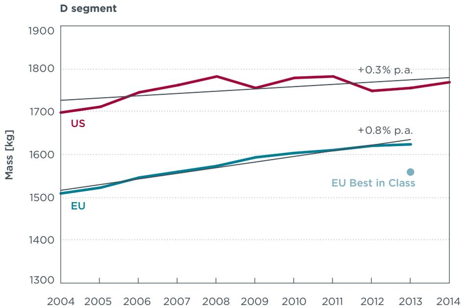
**Figure A-4.** Vehicle mass of D segment cars in the EU and U.S. - Annual averages of the past 10 years and actual best-in-class model.
