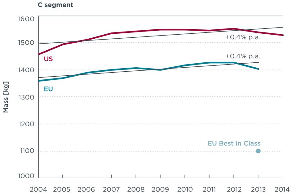
**Figure A-3.** Vehicle mass of C segment cars in the EU and U.S. - Annual averages of the past 10 years and actual best-in-class model.
