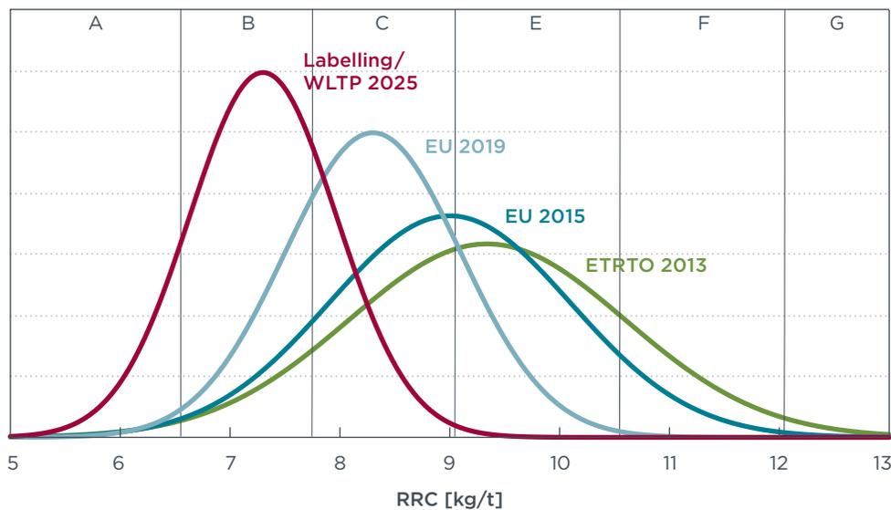
**Figure 14.** Projected development of tire rolling resistance distribution in the EU market for original equipment tires.
