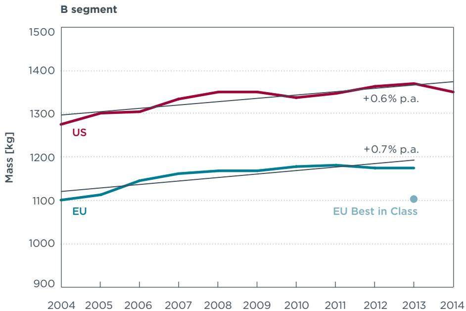
**Figure A-2.** Vehicle mass of B segment cars in the EU and U.S. – Annual averages of the past 10 years and actual best-in-class model.
