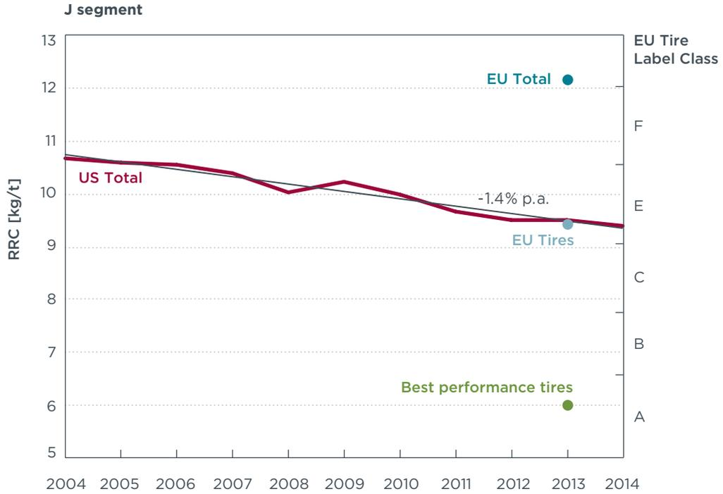
**Figure B-5.** Vehicle rolling resistance of J segment cars – Annual averages of the past 10 years in the U.S. and actual EU averages (total vehicle and tires only).
