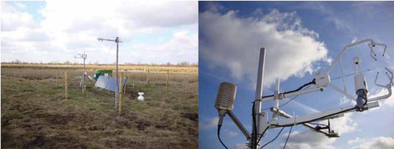
**Figure 8:** An eddy covariance flux tower measuring surface-atmosphere exchanges of CO<sub>2</sub>, water and energy at a restored fen peatland in the United Kingdom (left). Eddy covariance instrumentation, consisting of a sonic anemometer, an infrared gas analyzer, and sensors for measuring photosynthetically active radiation, air temperature and relative humidity (right). (Images: R. Morrison).
