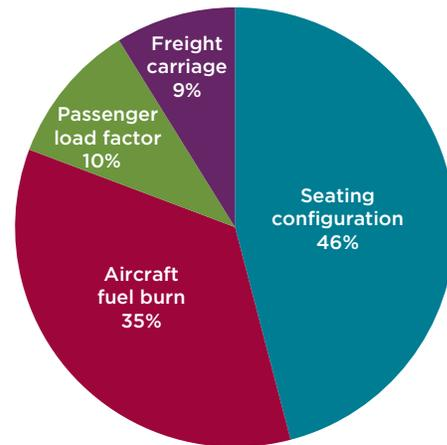
**Figure 3.** Key drivers of airline fuel efficiency
