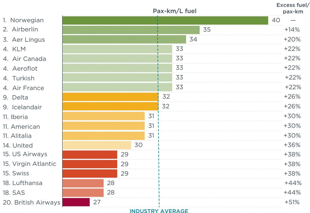
**Figure ES-1.** Fuel efficiency of the top 20 airlines on transatlantic routes, 2014
