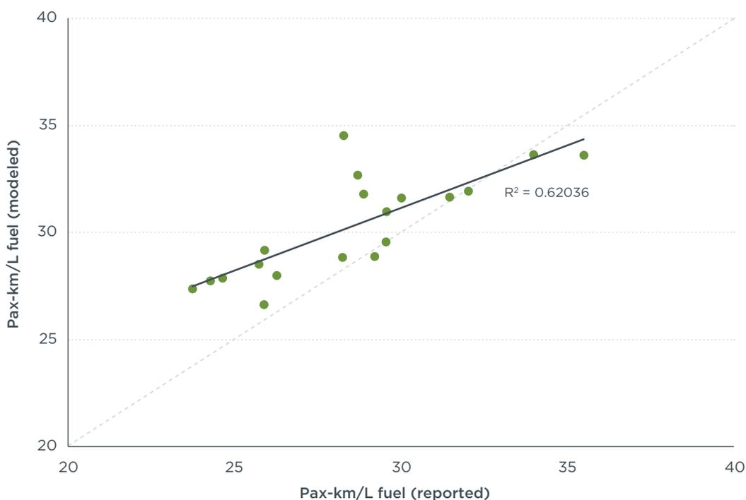
**Figure A3.** Airline-reported vs. modeled fuel efficiency
