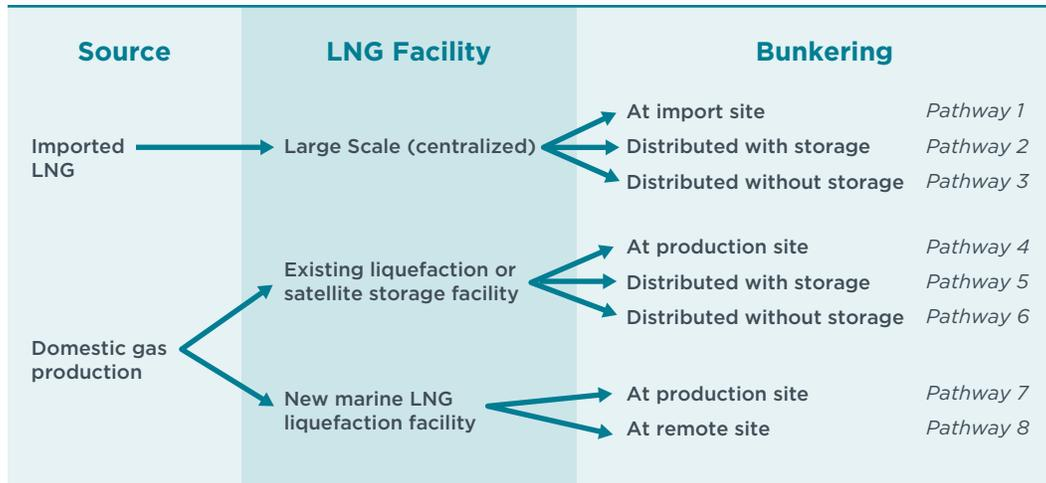
Figure 3: Analyzed LNG marine vessel bunkering pathways
