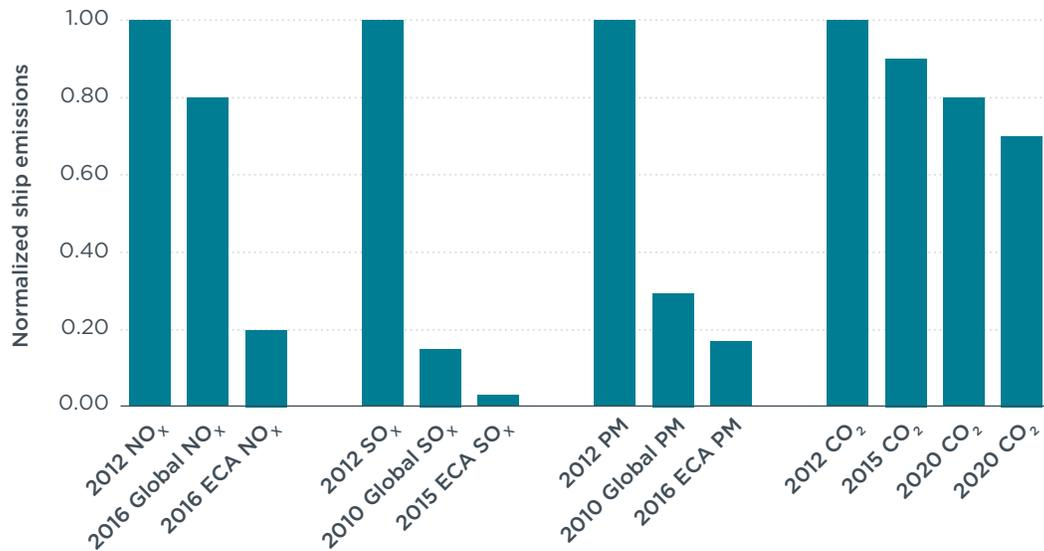
**Figure 2:** Required NO<sub>x</sub>, SO<sub>x</sub>, PM, and CO<sub>2</sub> emission reductions to meet new shipping vessel engine and fuel requirements in the 2015–25 time frame
