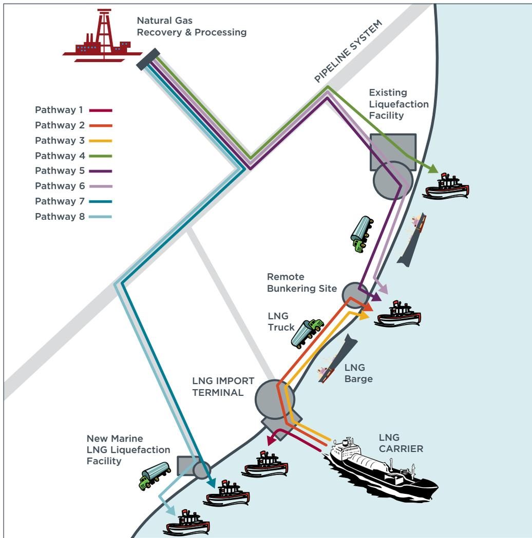
Figure 4: Illustration of LNG marine vessel bunkering pathways
