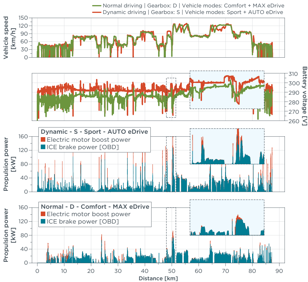
Figure 24. Effect of vehicle settings on the nonload voltage level setpoint of the high-voltage battery during real-world driving, starting with a depleted battery. For sports settings (gearbox in mode S and vehicle in sports mode), the battery voltage is increased to a nonload voltage of 295 V to support high propulsion power demands, while no charging is performed in normal mode (gearbox in mode D, vehicle in normal mode).
