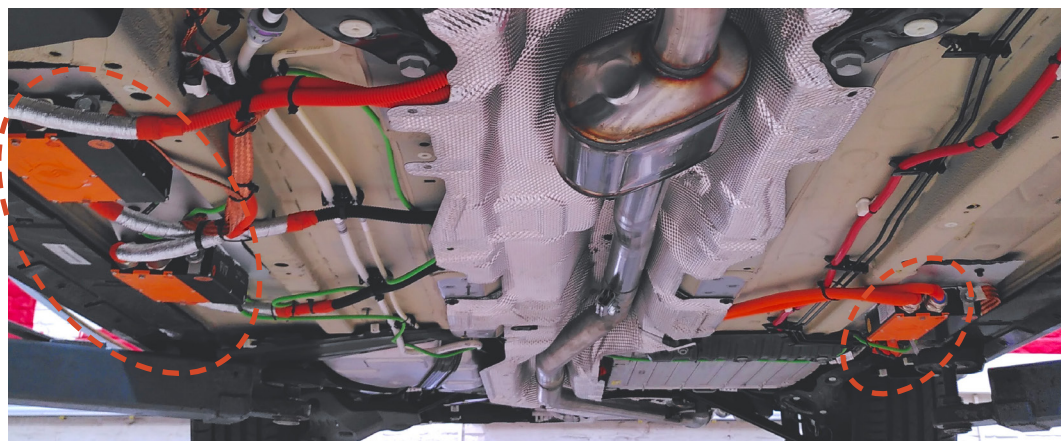
Figure 6. Installation of three high-voltage breakout modules in the test vehicle underfloor to measure energy flow at the high-voltage battery, air-conditioning compressor, and electric cabin heater.
