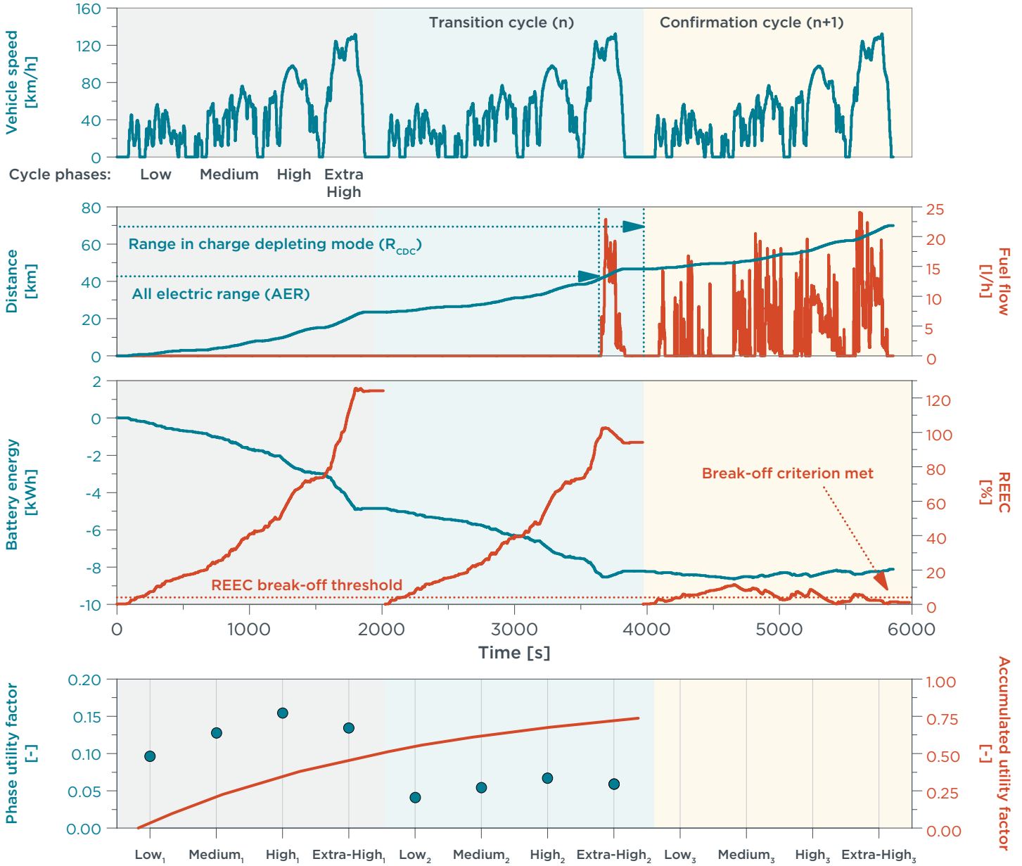
Figure 2. Principal of charge-depleting CO 2 emission determination. The top graph shows the speed profile of three WLTCs. Each cycle consists of phases low, medium, high, and extra-high. At the end of each test, the relative electric energy change (REEC) of the traction battery is calculated (right side of third graph from top). When the REEC drops below the break-off criterion of 4% at the end of a WLTC, charge-sustaining mode has been reached. This cycle is called the confirmation cycle and the preceding one the transition cycle. Only the cycles up to and including the transition cycle are considered being driven in charge-depleting mode. The left side of the bottom graph shows the utility factor used to weight each cycle phase until the end of the transition cycle. The accumulated utility factor (bottom graph, right side) is used to calculate the PHEV weighted, combined type-approval CO 2 emissions.
