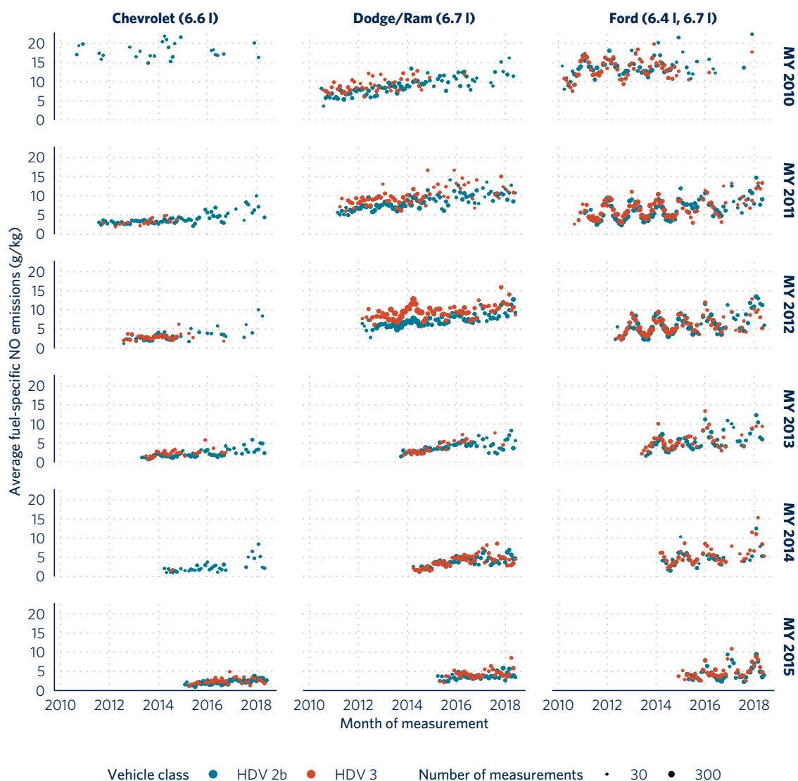
Figure 7. Average monthly fuel-specific NO emissions of three manufacturers and six model years of class 2b and class 3 diesel trucks.
