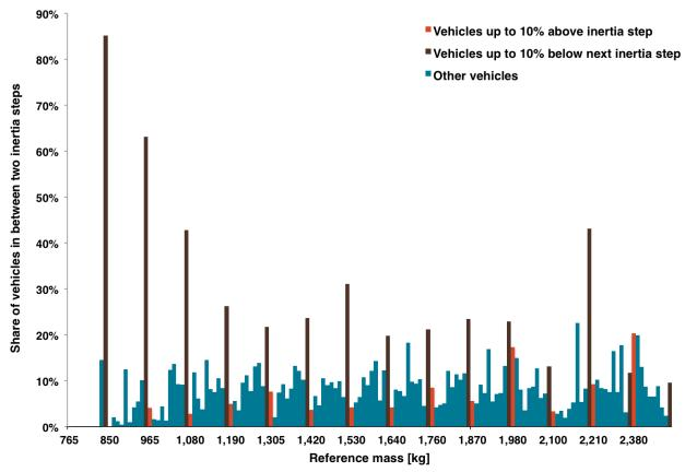
Figure 2. Distribution of new passenger car registrations by reference mass in EU-27 (2010) - Binned into 10 categories for each inertia class
