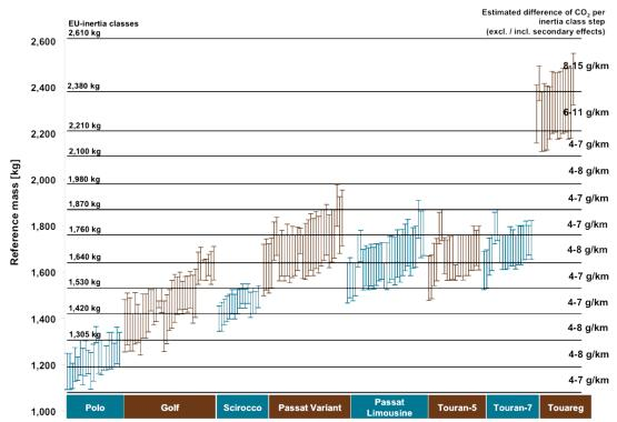
Figure 5: Vehicle weight ranges for some models of the Volkswagen passenger car fleet. Each line represents a vehicle version with the minimum and maximum reference mass, taking into account no/all available optional equipment
