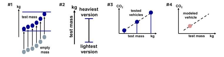
Figure 6. This 4-step approach would allow to change from the current inertia class based system to a step-less approach
