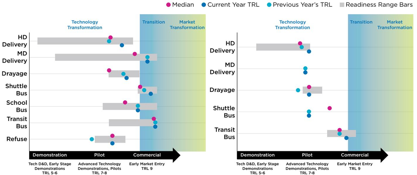
**Figure 4.** Technology readiness level (TRL) across major HDV market segments. Left: (a) on-road battery-electric powertrains. Right: (b) hydrogen fuel cell powertrains. Adopted from California Air Resources Board (2020).
