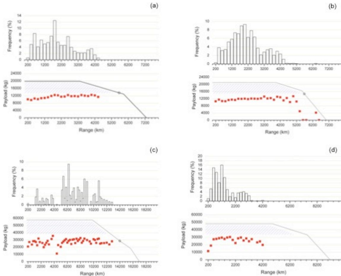
**Figure 4** Payload-Range diagrams with 200km incremental actual operational frequencies from BTS T100 data for (a) A320-200, (b) B737-800, (c) 777-200ER, and (d) A300-600 Freighter configuration for two major express freighter operators.
