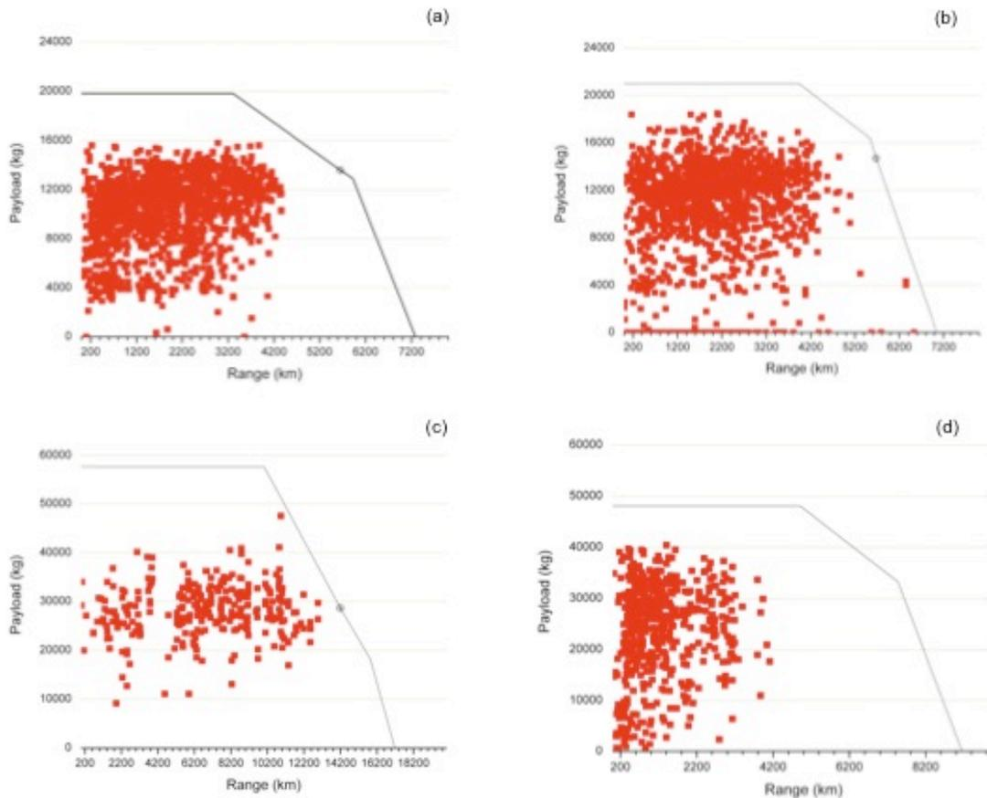
**Figure 3** Payload-Range Diagram for (a) Airbus A320-200, (b) Boeing 737-800, (c) Boeing 777-200ER, and (d) Airbus A300-600 Freighter for two major all freight operators. Red data points are point-to-point flights from BTS T100 data for December 2006.<sup>5</sup>
