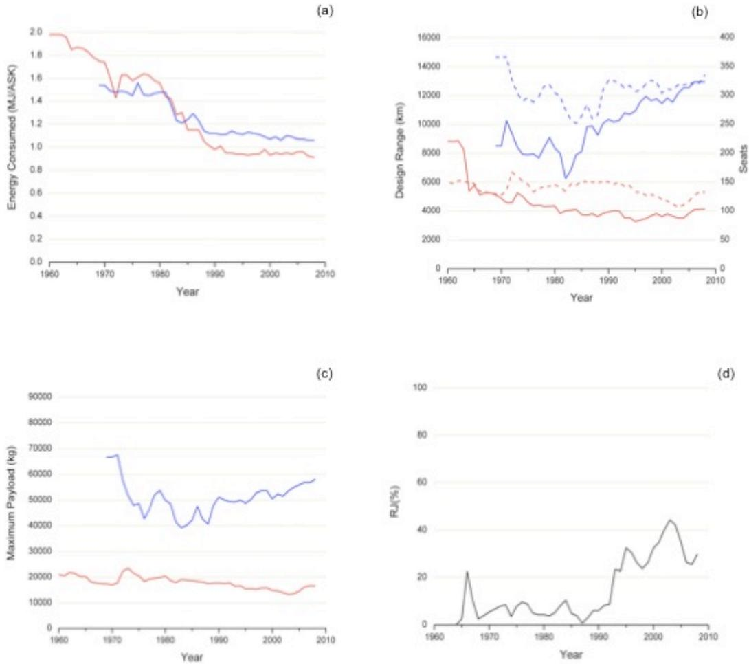
**Figure 1** Historical trends for newly delivered aircraft. (a) Estimated energy consumption at design payload and range left axis,(b) Range at design payload, solid lines left axis; estimated number of available seats, dashed lines right axis, (c) Maximum payload, and (d) Regional jet deliveries. For all: Red lines narrowbody, blue lines widebody.
