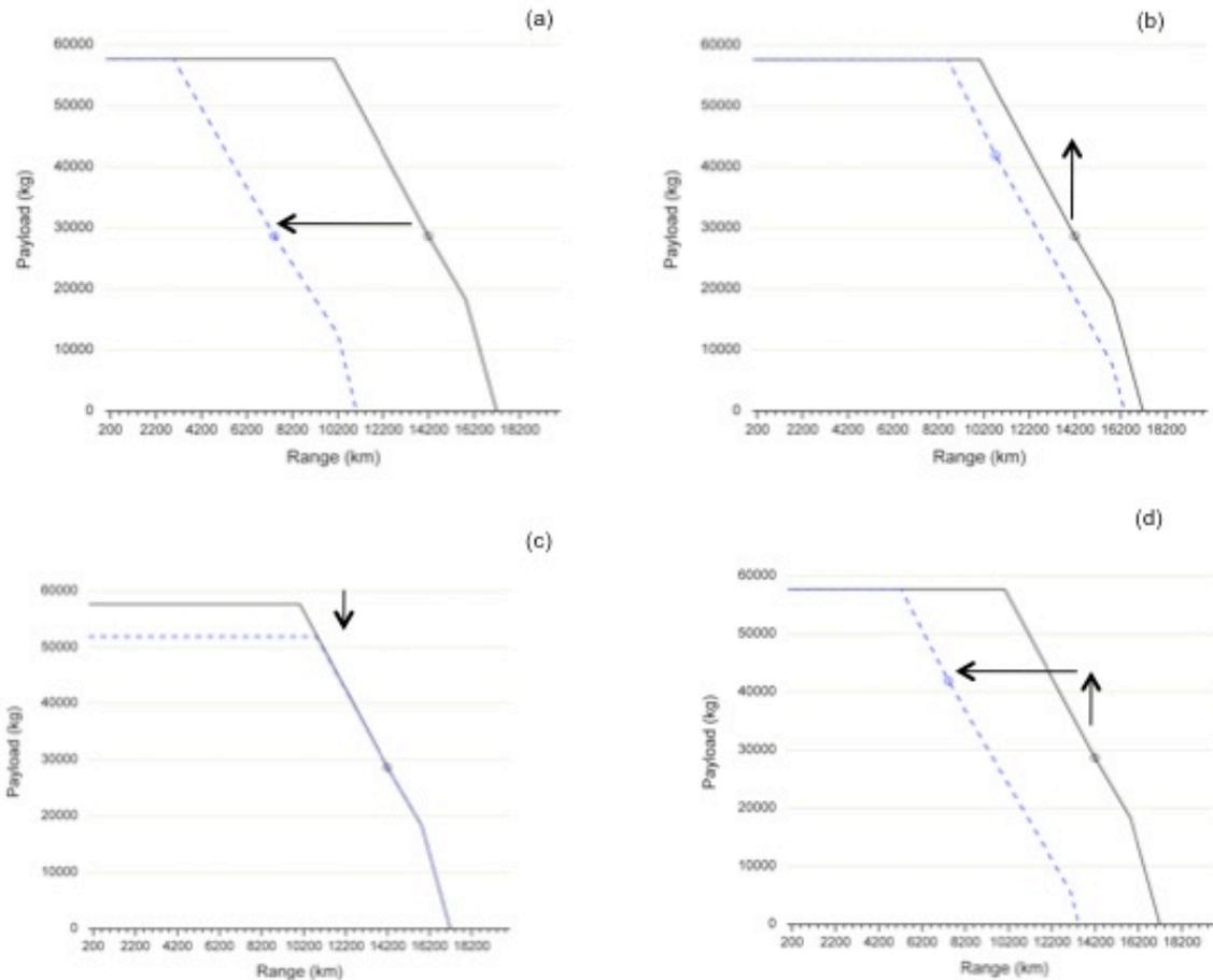
**Figure 6** Schematic representation of variation in payload-range (a) nominal design range change, (b) nominal design payload change, (c) maximum payload reduction, and (d) both increase design payload and decrease in range change.
