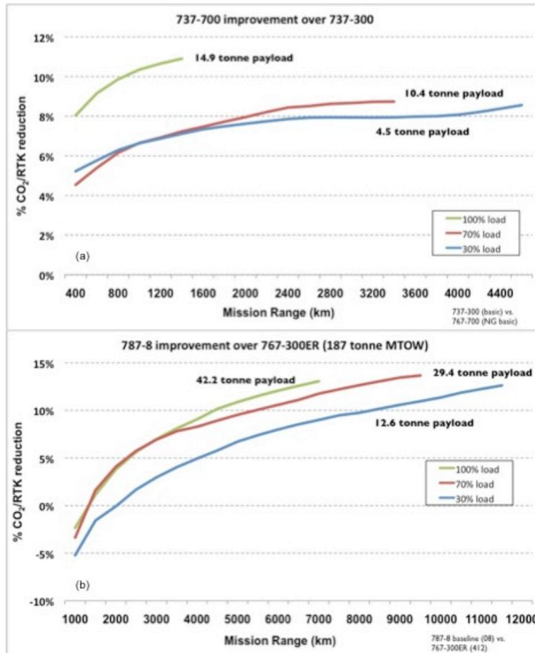
**Figure 5** Relative block CO<sub>2</sub> intensity reductions by mission range and payload for (a) B737-700 v. 737-800 and (b) 787-8 v 767-300ER.
