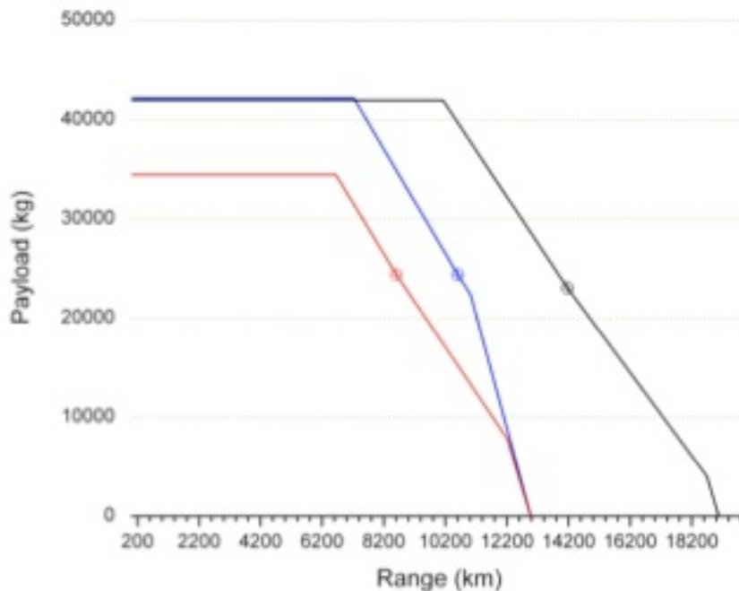
**Figure 2:** 767-300ER vs. 787-8 payload/range diagrams. Lines: black B787-8, blue b767-300ER(187 tonne), and red B767-300ER(172 tonne). Crossed circle denotes nominal design payload and range. All parameters at default Piano values.
