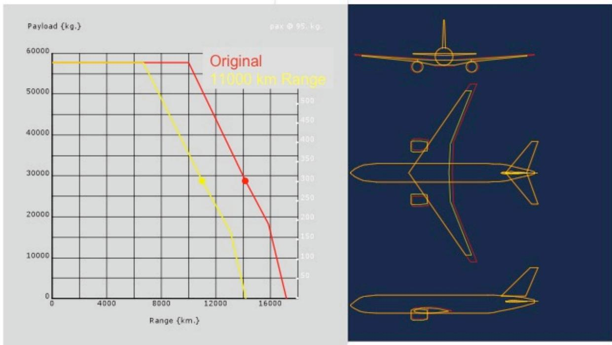
**Figure A 1** Payload-Range diagram and 3-view profile for B777-200ER range re-size.
