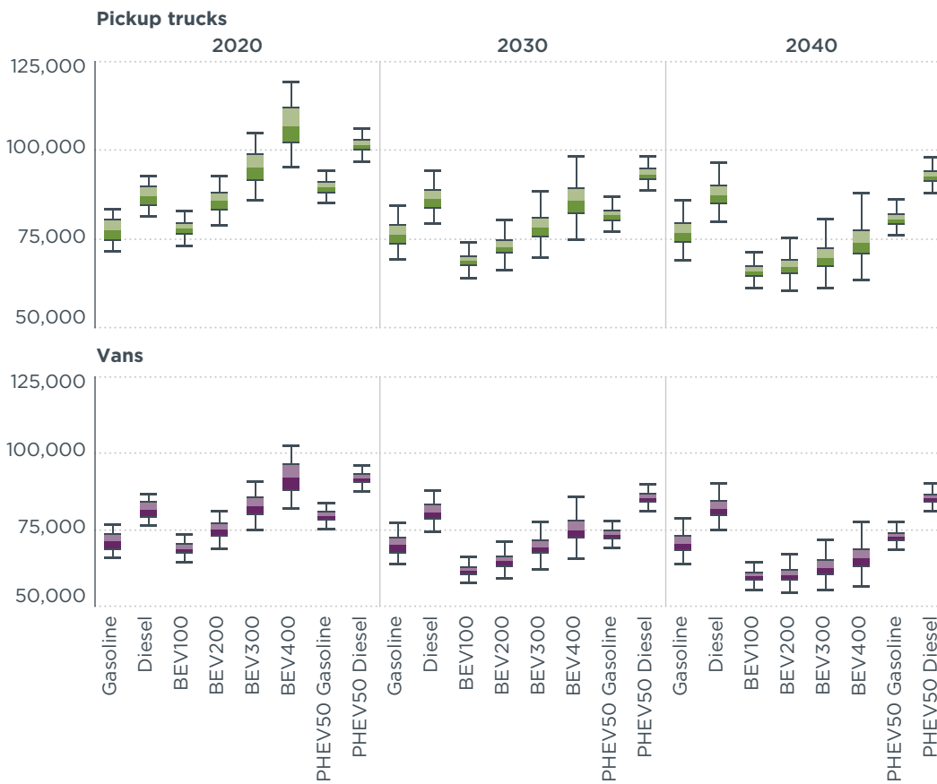
Figure 9. Sensitivity analysis of TCO values for pickup trucks and vans across 2020, 2030, and 2040.
