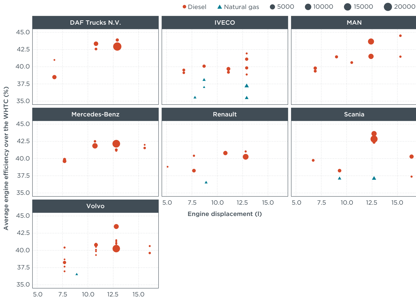
Figure 9. Calculated cycle-averaged engine efficiency (WHTC) for the top-selling manufacturers. Each engine's specific combination of displacement and rated power is associated with an engine model. The size of the points represents the number of trucks equipped with each engine model.
