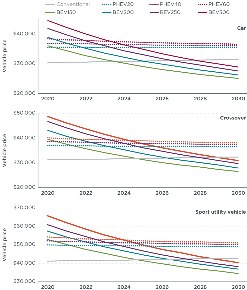
Figure 4. Initial purchase price of conventional and electric cars, crossovers, and SUVs for 2020-2030.
