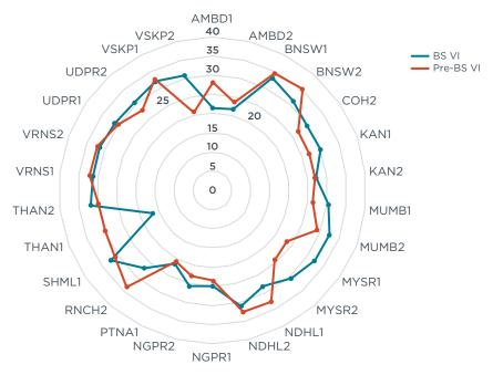
Figure 18. Aromatics comparison between pre-BS VI and post-BS VI samples.
