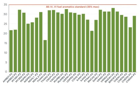
Figure 4. Aromatics content analyzed in all gasoline samples.
