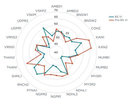
Figure 17. RVP comparison between pre-BS VI and post-BS VI samples.
