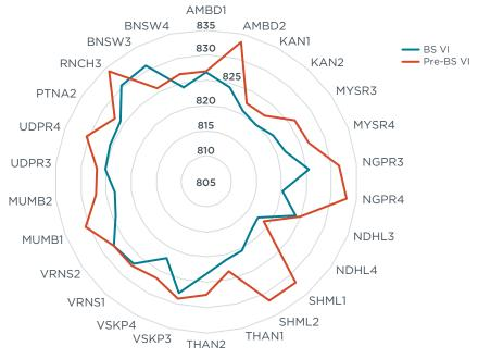
Figure 24. Density comparison between pre-BS VI and post-BS VI samples.
