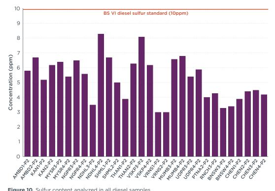
Figure 10. Sulfur content analyzed in all diesel samples.
