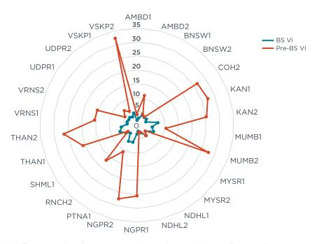
Figure 21. Sulfur comparison between pre-BS VI and post-BS VI gasoline samples.
