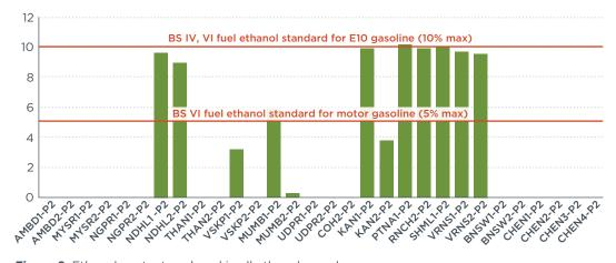
Figure 8. Ethanol content analyzed in all ethanol samples.
