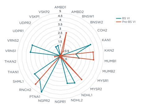
Figure 23. Oxygen content comparison between pre-BS VI and post-BS VI samples.
