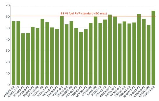
Figure 2. RVP analyzed in all gasoline samples.
