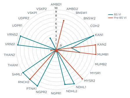
Figure 22. Ethanol content comparison between pre-BS VI and post-BS VI samples.
