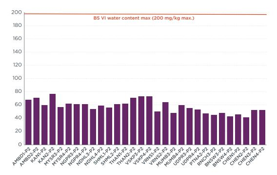
Figure 14. Water content analyzed in all diesel samples.
