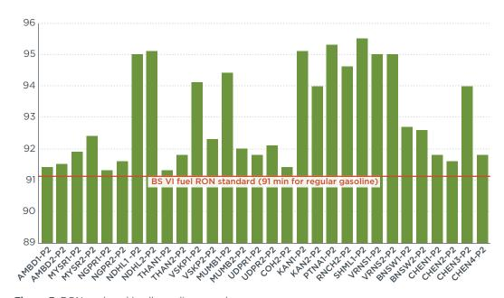
Figure 3. RON analyzed in all gasoline samples.
