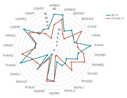
Figure 19. Olefins comparison between pre-BS VI and post-BS VI samples.
