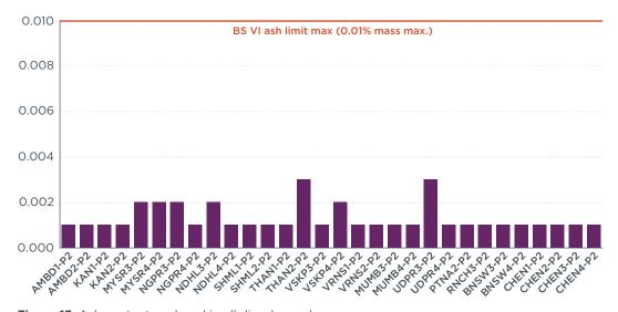
Figure 13. Ash content analyzed in all diesel samples.
