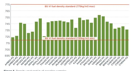
Figure 5. Density analyzed in all gasoline samples.
