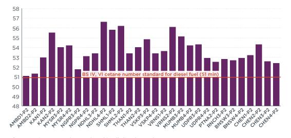
Figure 11. Cetane number analyzed in all diesel samples.
