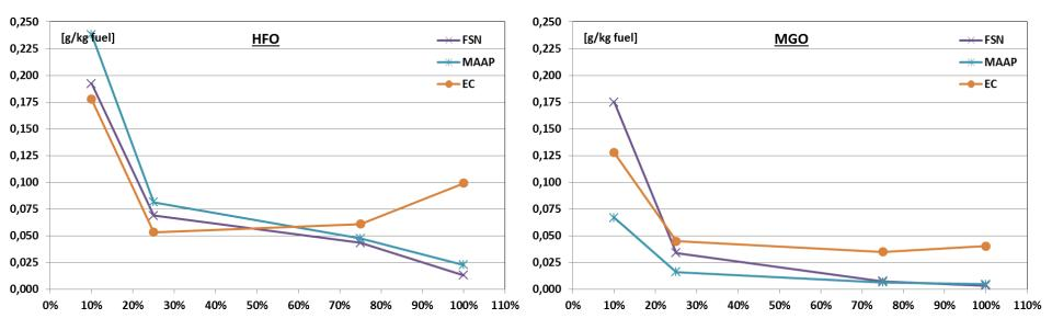
Resulting BC emission factor for medium speed 32/44 diesel engine, mean ±standard deviation of all FSN & MAAP & in-house EC for HFO & MGO, is <u>0.069±0.065</u> (24 points) -> Is such a single value of any significance?
