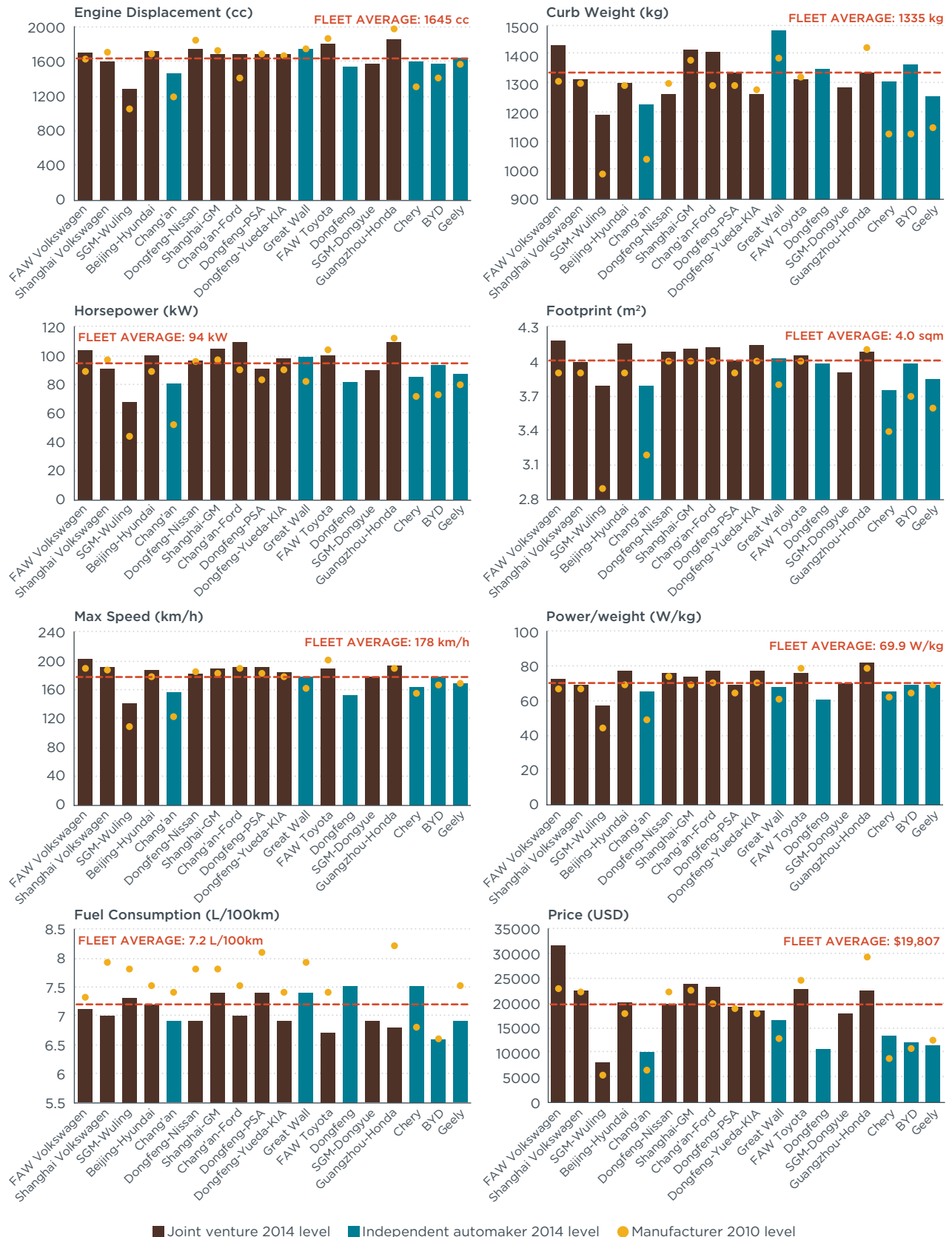
Figure 3.2.2 Averages of key parameters by top-selling manufacturers (independent automakers vs. joint ventures)
