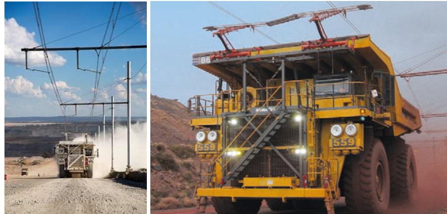
Figure 24 Mining trucks under a catenary
