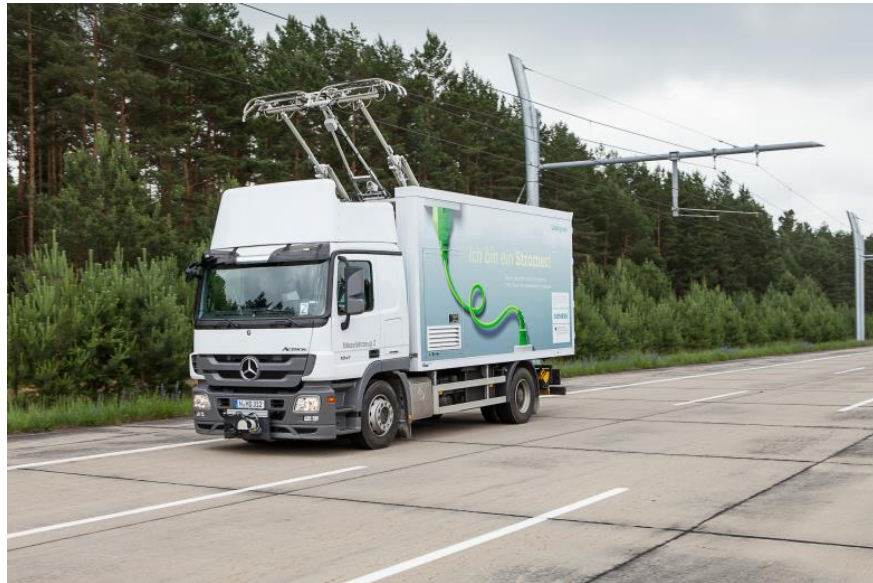
Figure 22 Hybrid Truck under a catenary
