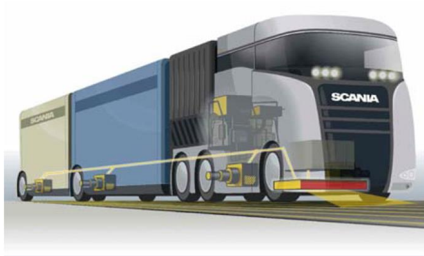
Figure 19 Hybrid truck with electric drivetrain of Scania that is used in the inductive charging demonstration project
