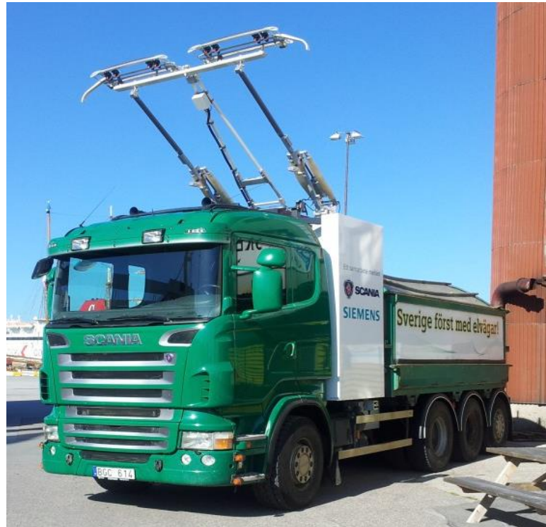
Figure 23 Overhead catenary prototype truck by Scania and Siemens
