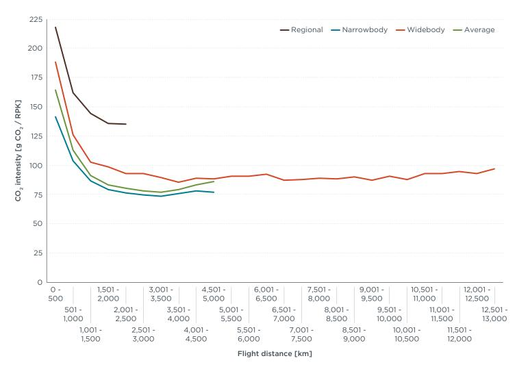
**Figure 10.** Passenger  $CO_2$  intensity in 2019, by stage length and aircraft class
