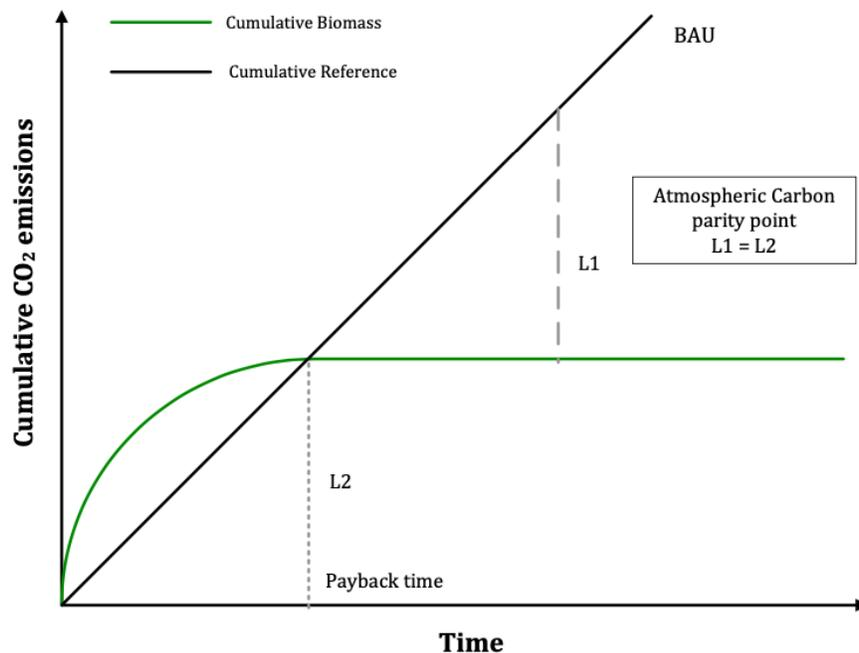
Figure 5: Visual description of payback time and atmospheric carbon parity point. Green Line: drop in the forest carbon stock due to bioenergy production; Black line: accumulated reduction in carbon emissions from substitution of fossil fuels. Source: [4]
