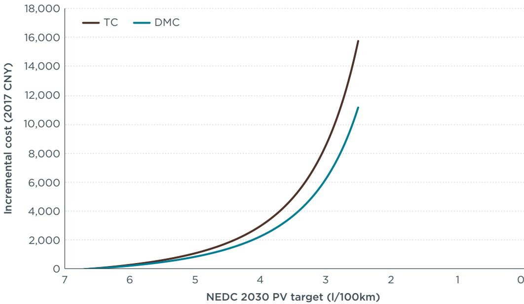
**Figure ES2.** 2030 NEDC fuel consumption incremental compliance costs for passenger vehicles under ICE strategy.
