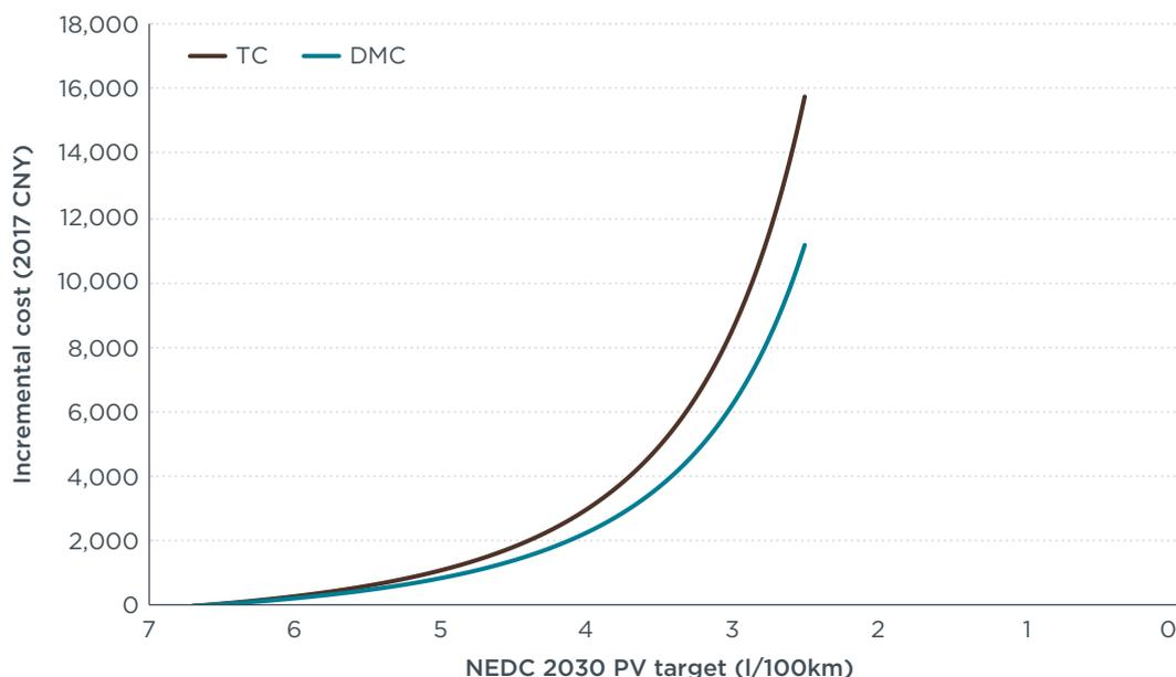
**Figure 4.** 2030 NEDC fuel consumption incremental compliance costs for passenger vehicles under ICE strategy.
