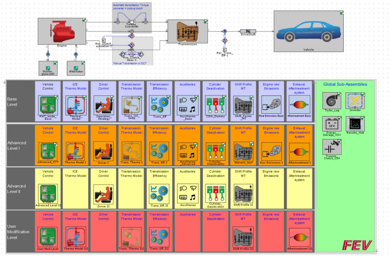
Figure 2. FEV GT-Suite Simulation Model (FEV, 2015).
