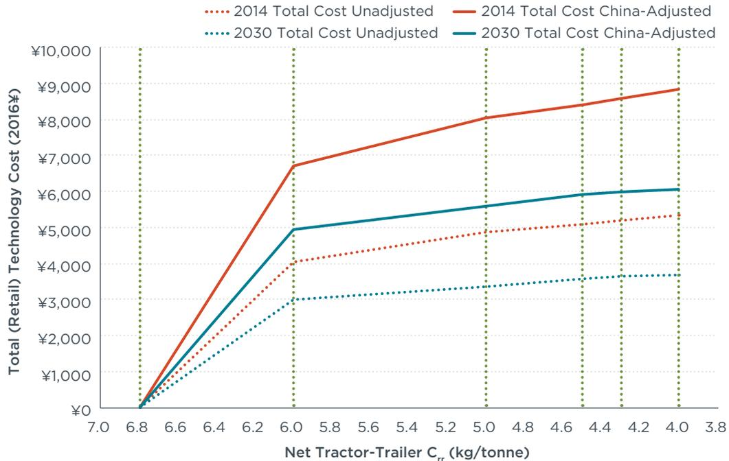
**Figure 7.** Rolling resistance technology cost curves (1.045 trailers per tractor)
