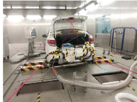
Figure 7. PEMS verification on chassis
