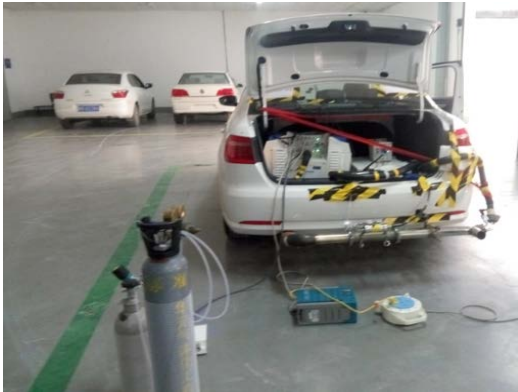
Figure 6. PEMS installation dynamometer
