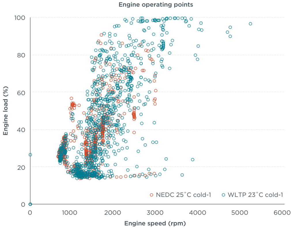
Figure 21. Engine operating points of Vehicle 32 over NEDC and WLTP
