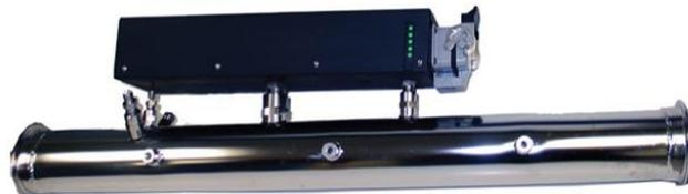
Particulates were measured by a Pegasor Mi2, which is a real-time sampler of the raw exhaust. It uses a corona diffusion charger for estimating both particle number and mass. It can be configured to measure either particle mass concentration or number concentration. It is an alternative method to the filter-paper-based regulatory approach, but has the advantages that:
