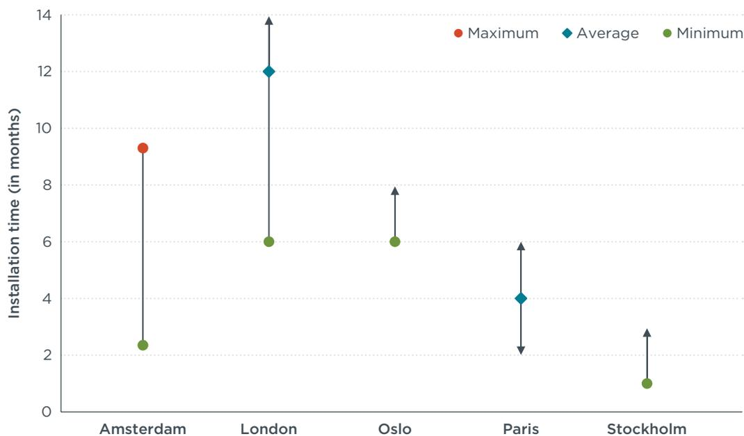
**Figure 1.** Time needed to install an AC regular charging station in selected cities.
