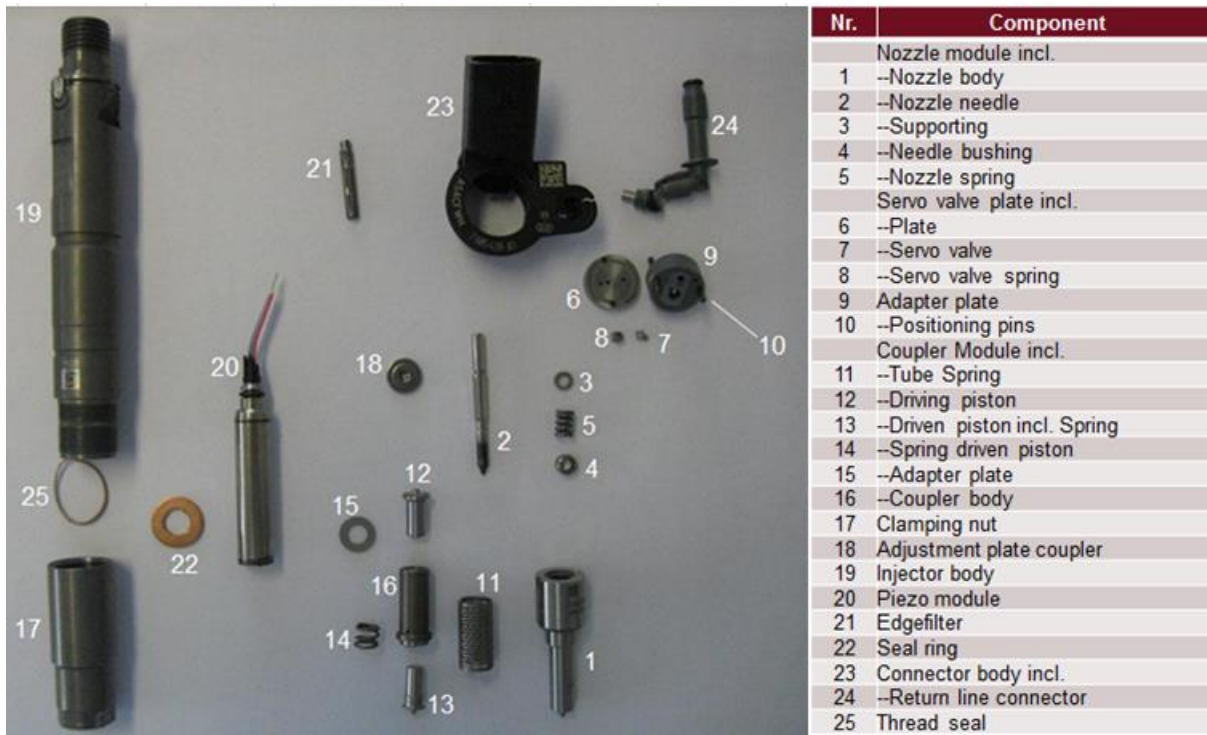
Figure B-3: Initial Level of Injector Teardown
