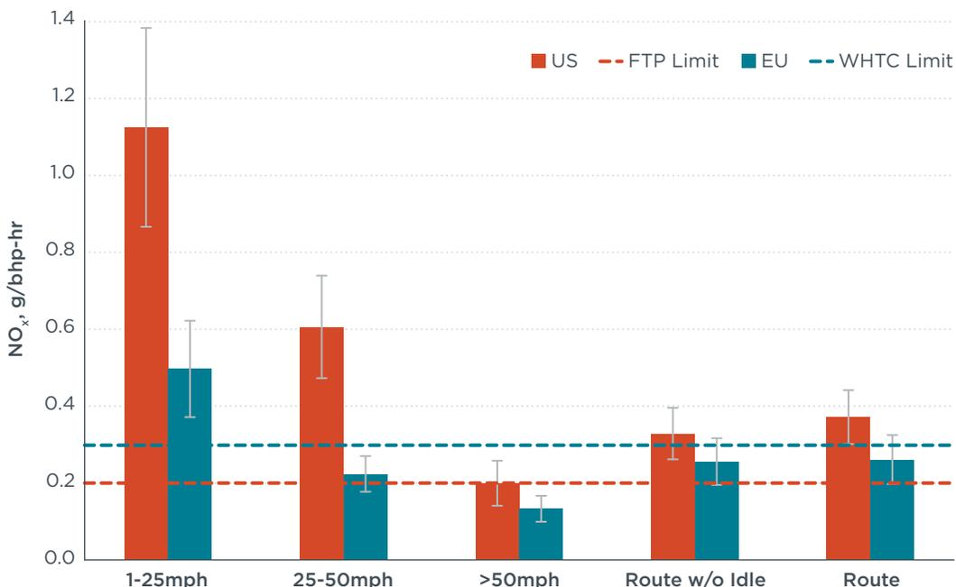
NO<sub>x</sub> emissions by speed bin for European and U.S. heavy-duty vehicles. Dotted lines represent engine emission NO<sub>x</sub> limits defined by U.S. (as measured on the Federal Test Procedure) and European (World Harmonized Transient Cycle) HDV emissions regulations.
