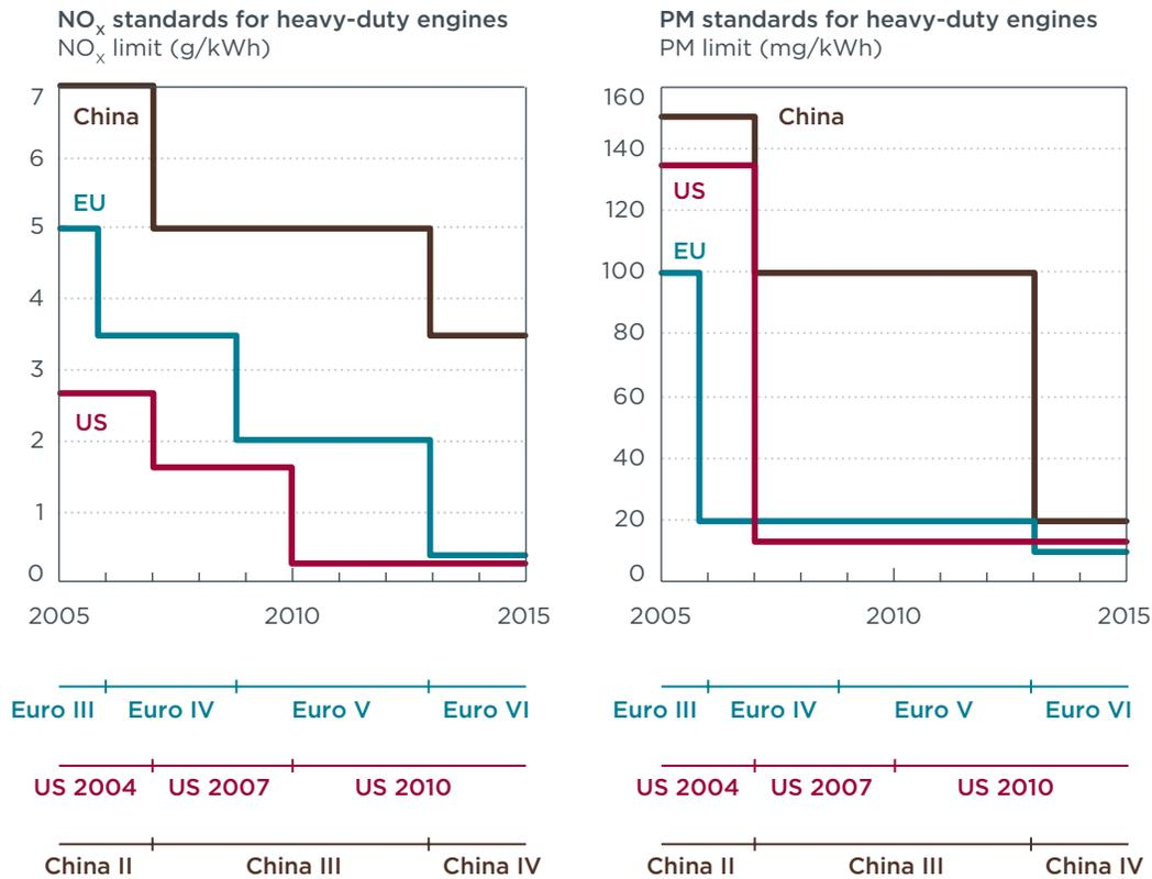
**Figure 14.** NO<sub>x</sub> and PM emission limits for new type approvals in the EU, U.S., and China.\*
