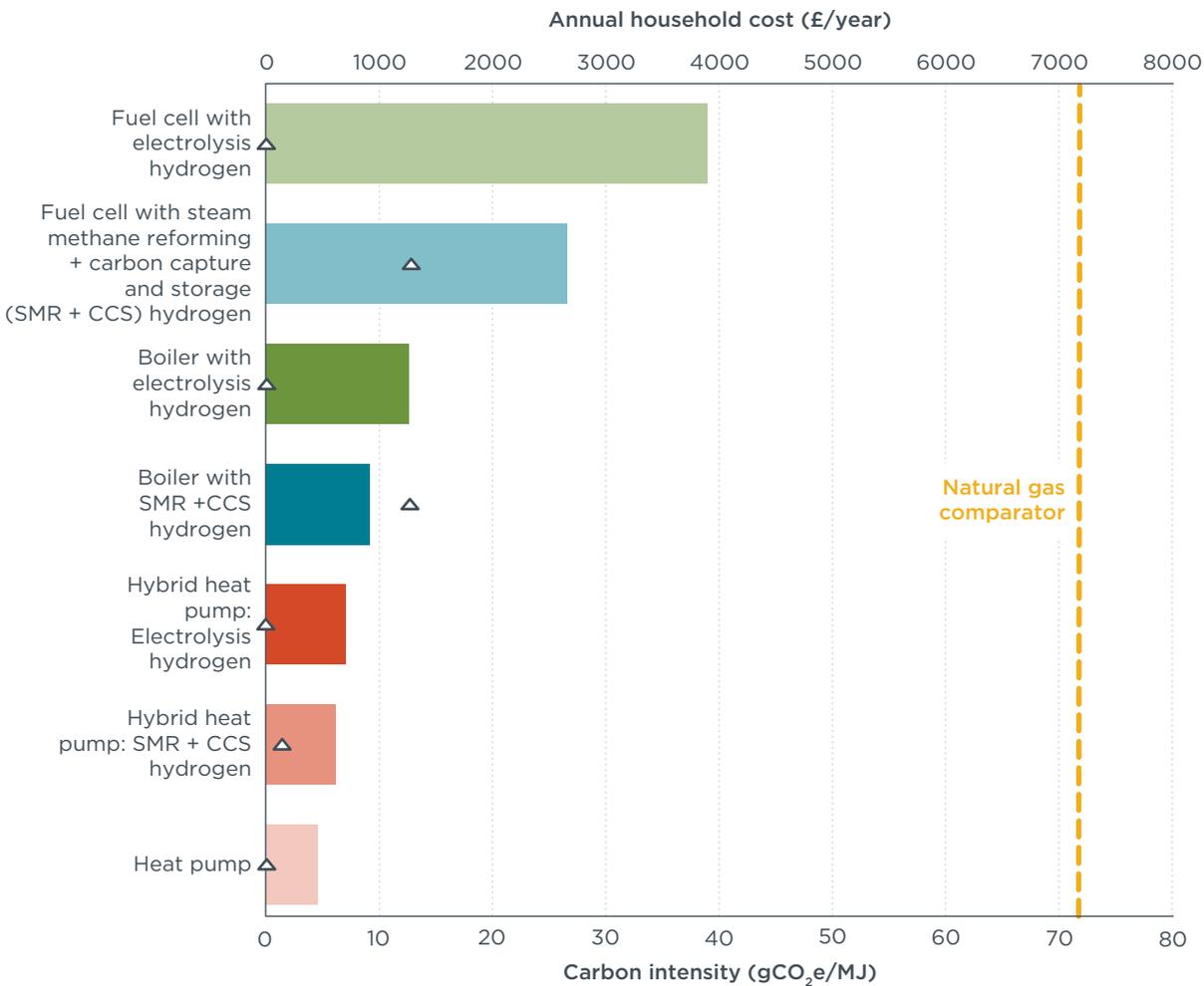
**Figure 1:** Cost comparison and carbon intensities of different technology options for heating a household for one year in the United Kingdom in 2050. Triangles represent the carbon intensity of the different pathways along with a natural gas comparator.
