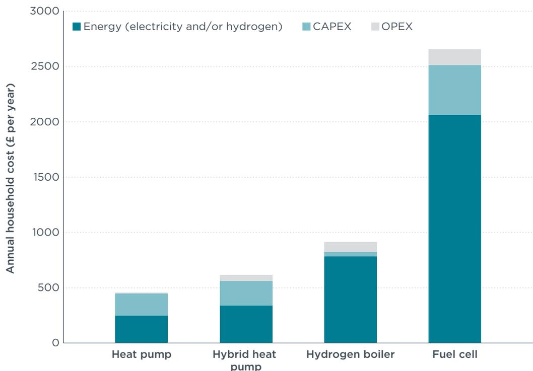
**Figure 3:** Cost components of heating pathways. Note: The cost of energy for the fuel cell scenario is net of excess electricity generation that is sold to the grid. For the pathways using hydrogen, the hydrogen is from SMR + CCS.
